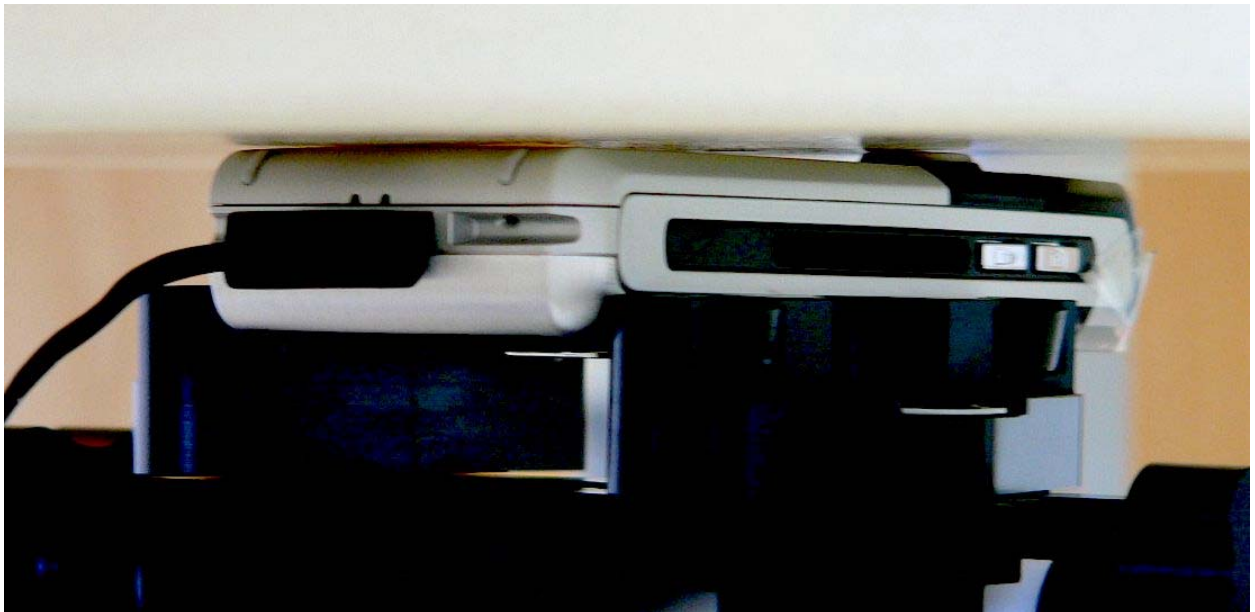
Fig. 30: Body worn configuration Siemens SXG75, GSM mode with headset, antenna towards the phantom, gap= 0 mm.
