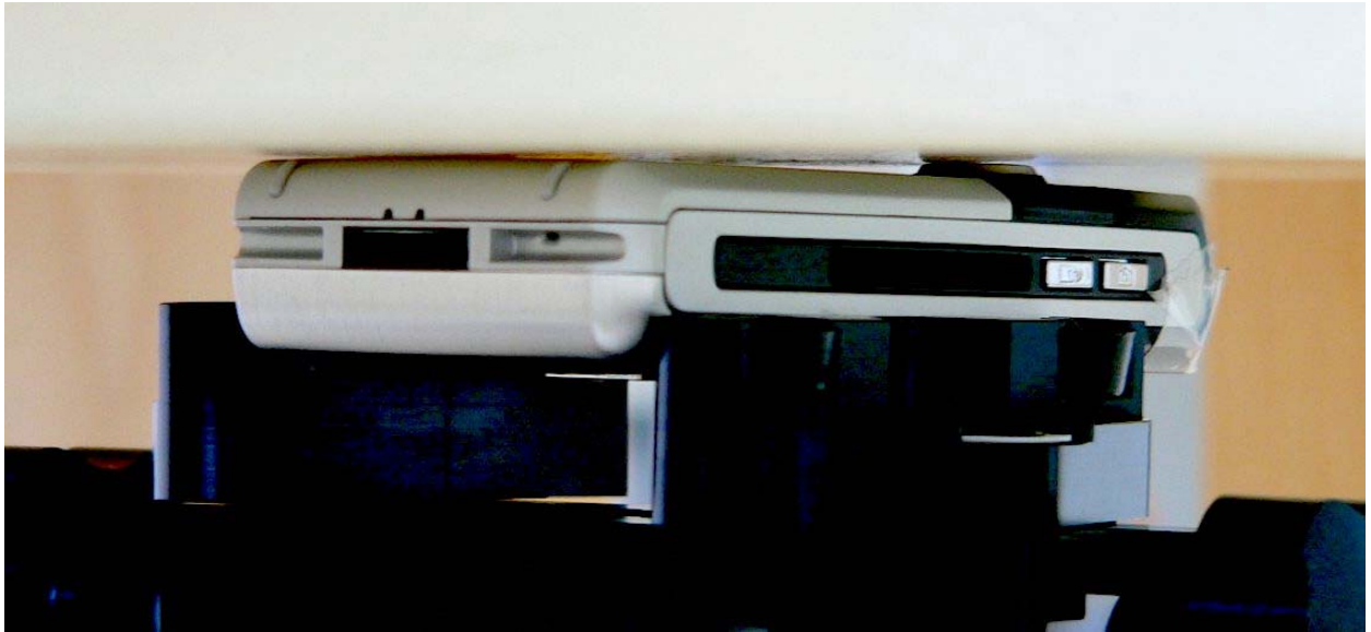
Fig. 29: Body worn configuration Siemens SXG75, GSM mode, without accessory, antenna towards the phantom, gap= 0 mm.
