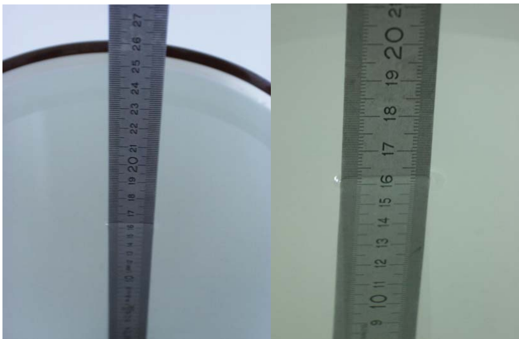
Fig. 33: Liquid depth for PCS 1900 Head and Body measurements.
