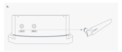
Insert LTE antenna 2 into LTE antenna 2 port and rotate the antenna nut in a clockwise direction until it is firm. Ensure not to overtighten.
