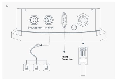
Connect machine's RJ45 ethernet male connector to the RJ45 female port of Phantom Edge and rotate connector nut in a clockwise direction to tighten it
