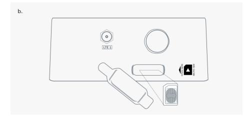
Insert Micro SIM into Phantom Edge as per the marking sticker
