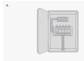
Identify the MCB switch associated with relevant electrical load/machine
