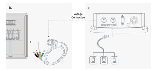
Remove approx. 50mm of insulation from wires. Connect the four-individual wire strands in the voltage connector cable to the appropriate points of the four-pole MCB. Follow color coding of the wire strands to ensure correct connection (*Refer exhibit 1*). Connect the female connector of this cable to the male connector on Phantom Edge, which is labelled as Voltage Input
