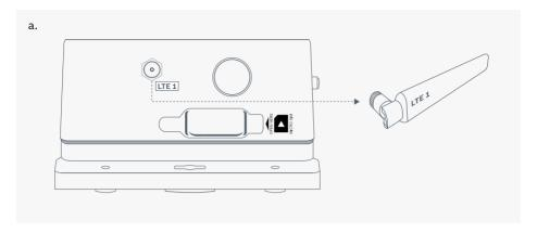
Insert LTE antenna 1 into LTE antenna 1 port and rotate the antenna nut in a clockwise direction until it is firm. Ensure not to overtighten.
