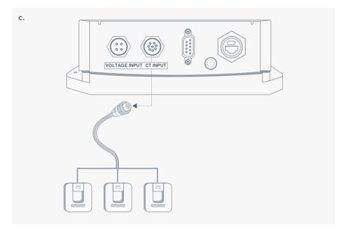
Connect the CT female connector to the male connector on Phantom Edge, which is labelled as Current Input
