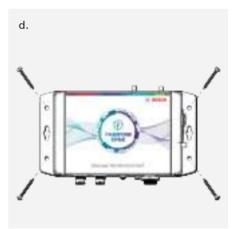
Mount the Phantom Edge on the wall using the four screws provided in the kit
