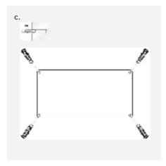
Insert four wall plugs into the drill holes with the help of hammer
