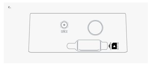
Close the Micro SIM cap and fasten it firmly without any bulge
