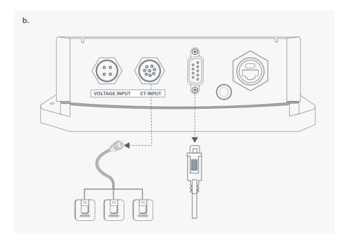
Connect machine PLC RS232 female connector to the male connector of Phantom Edge and tighten the screws
