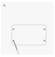
Drill holes of sufficient depth to accommodate wall plugs provided in the installation kit
