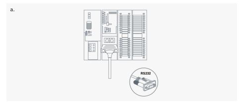
Identify RS232 female connector connected to machine PLC
