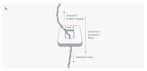
Clamp CT around the individual power cable for each phase. Ensure that the front surface of the CT and line label, is oriented in the direction of power source. Ensure color code of the power cable and line label matches. (*Refer Exhibit 1*)
