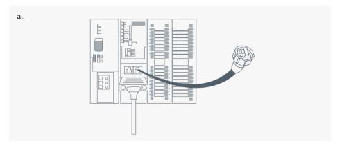
Identify the recommended Amphenol RJ45 Cable RCP-5SAMMM-SLM7Bxx male connector connected to machine PLC
