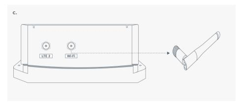
Insert Wi-Fi antenna into Wi-Fi antenna port and rotate antenna nut in a clockwise direction until it is firm. Ensure not to overtighten.
