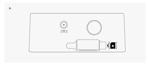
Gently pull the flap on its right side to reveal the Micro SIM card slot
