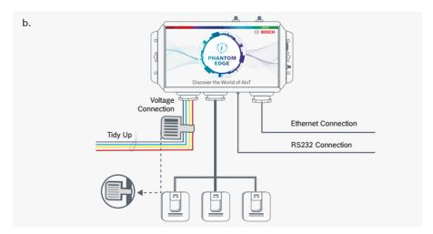
Fill in the contact details of local technician and tag it on the voltage cable. Ensure all details are correctly filled for emergency response.
