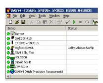
Most of the DASY items and requirements do not deviate from those for the frequency range below 3 GHz. However, due to the stronger gradients of the field distribution in the 5-6 GHz frequency range, adaptation is required for the scanning method as well as for the dosimetric probe type.
