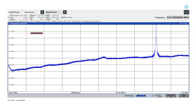
The peak above the limit is the carrier frequency: LTE Band 26, 824 MHz
