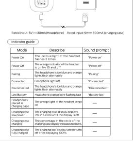
Connect the charging case to the 5V power adapter with Type-C charging cable.
