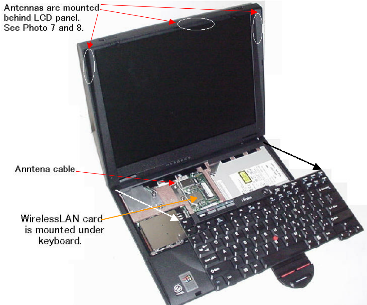
Photo.5: Locations of IEEE802.11b Wireless-LAN mini-PCI card and Antenna
