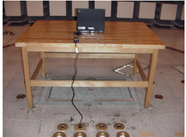
Radiated Emission – Rear View (EMI SEMIANECHOIC CHAMBER)
