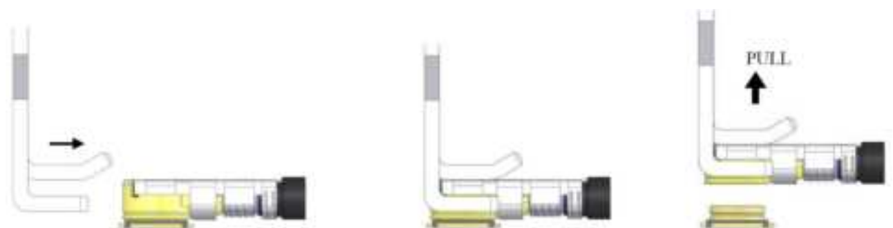
Figure 4-7 Lift up pulling JIG
