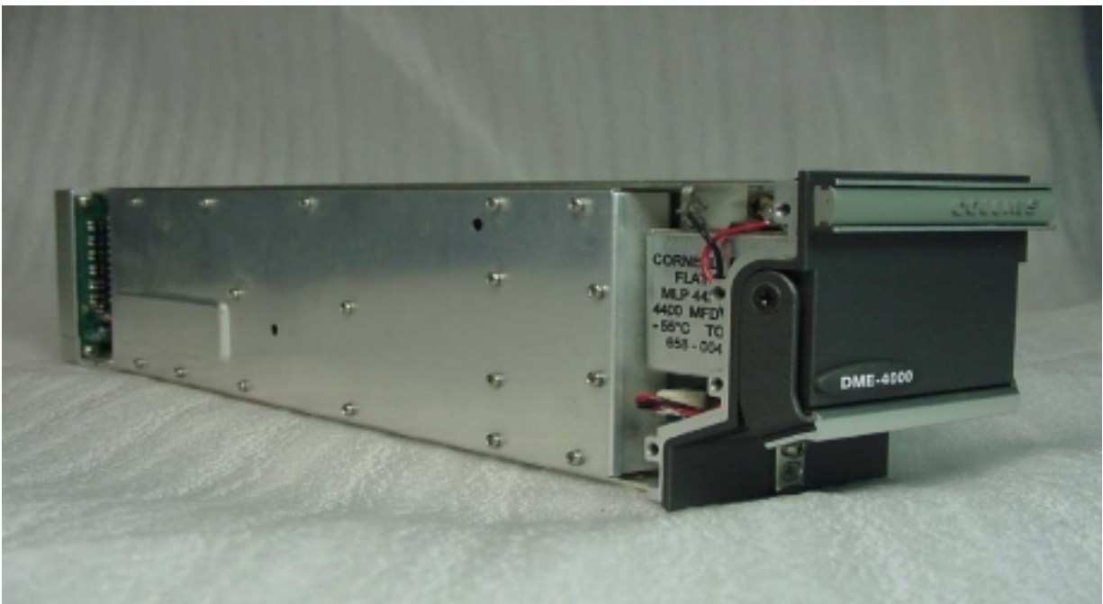
The DME-4000 Modulator/IF/Synthesizer side of the unit with the unit cover removed and the Modulator/IF/Synthesizer cover exposed. Partial view of the storage capacitor behind the front panel.
