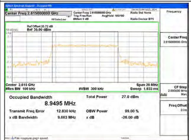
B38 / 10MHz / 16QAM/ High CH
