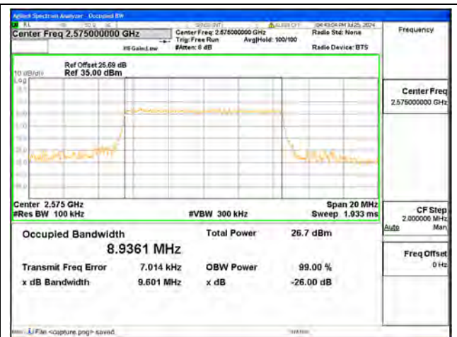
B38 / 10MHz / 16QAM/ Low CH
