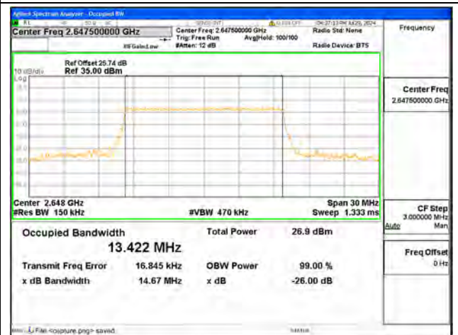
B41 / 15MHz / 16QAM/ High CH
