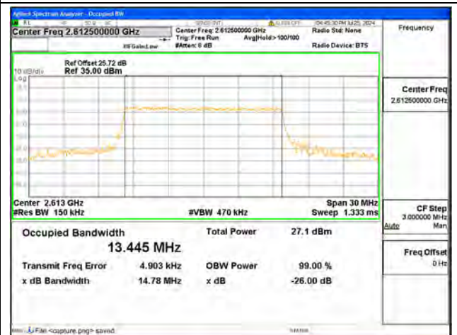
B38 / 15MHz / 16QAM/ High CH
