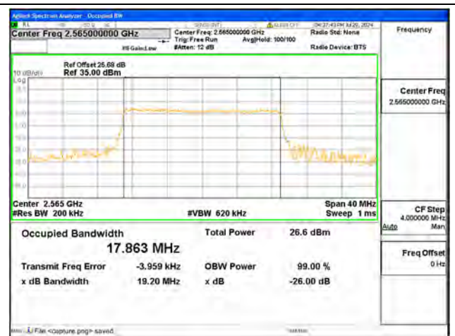
B41 / 20MHz / 16QAM/ Low CH
