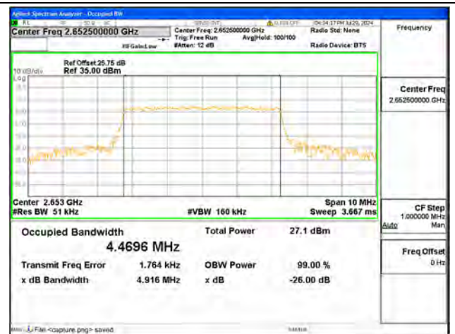
B41 / 5MHz / 16QAM/ High CH
