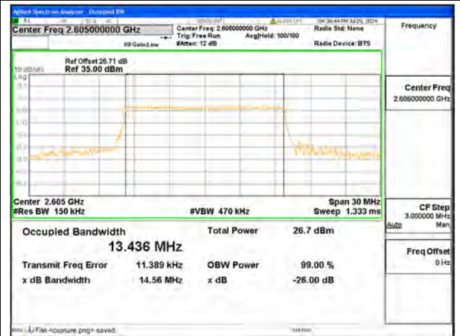
B41 / 15MHz / 16QAM/ Mid CH
