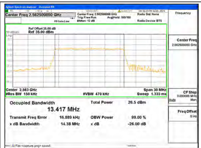
B41 / 15MHz / 16QAM/ Low CH
