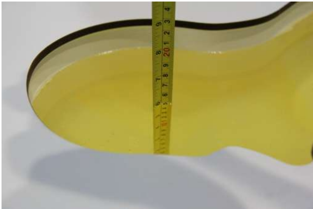
Picture 7-5: Liquid depth in the Head Phantom(2450MHz)
