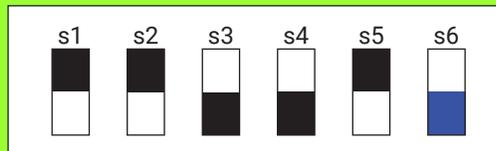
**Figure 67: RMC Dip Switch Example - 13 dB in Normal Mode**
