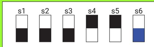
**Figure 62: RMC DIP Switch Example - 8 dB Normal Mode**
