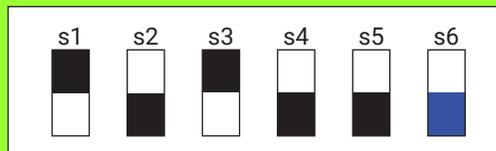
**Figure 81: RMC Dip Switch Example - 27 dB in Normal Mode**
