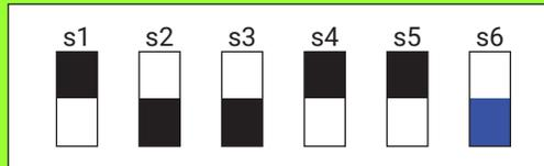
**Figure 61: RMC DIP Switch Example - 7 dB Normal Mode**
