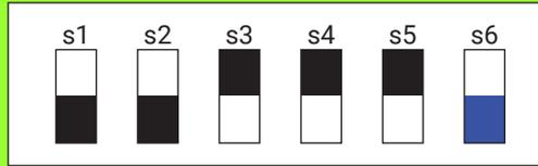
**Figure 58: RMC DIP Switch Example - 4 dB Normal Mode**
