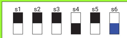
**Figure 63: RMC DIP Switch Example - 9 dB Normal Mode**
