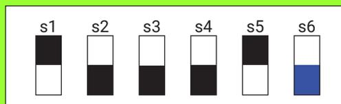
**Figure 69: RMC Dip Switch Example - 15 dB in Normal Mode**
