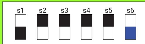
**Figure 56: RMC DIP Switch Example - 2 dB Normal Mode**
