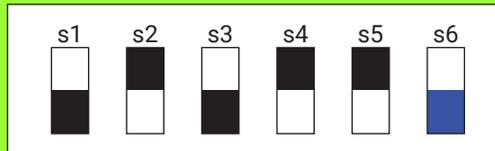
**Figure 60: RMC DIP Switch Example - 6 dB Normal Mode**
