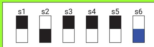
**Figure 57: RMC DIP Switch Example - 3 dB Normal Mode**
