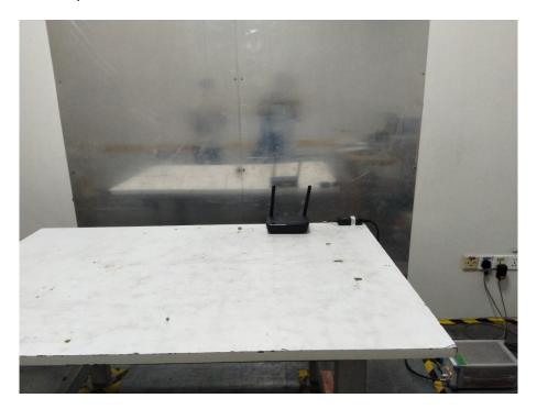
Radiated Spurious Emissions(30MHz-1GHz)
