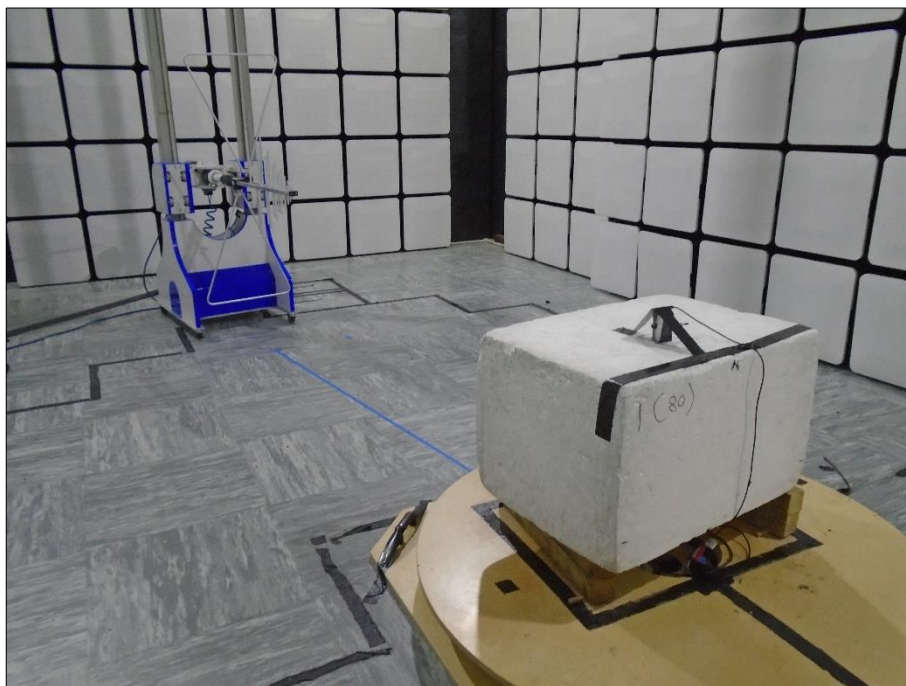
Figure 141 - Test Setup - 30 MHz to 1 GHz Y Plane
