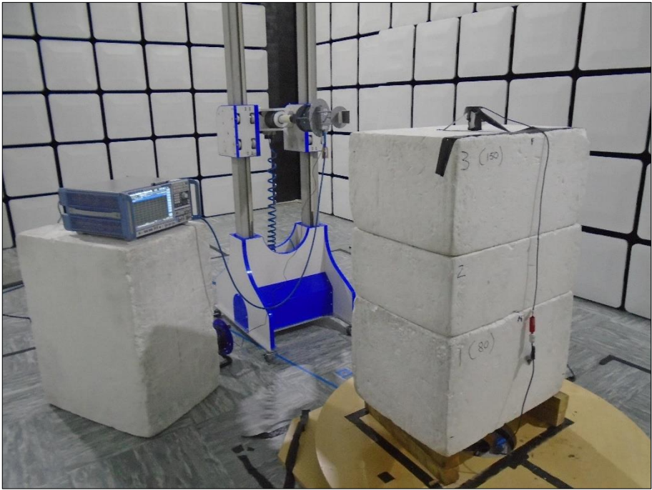
Figure 147 - Test Setup - 18 GHz to 25 GHz Y Plane
