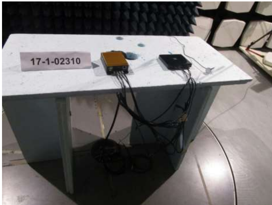
Figure 7: Close View 9 KHz – 30 MHz EUT Laying
