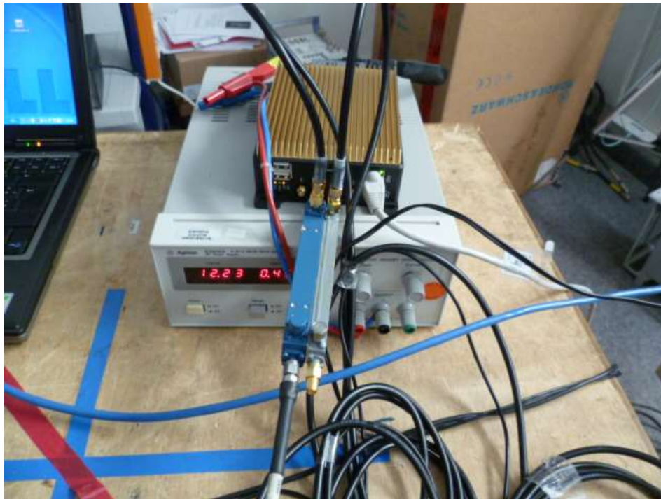
Figure 3: μCROS SL Close View Conducted Sample for WLAN Testing
