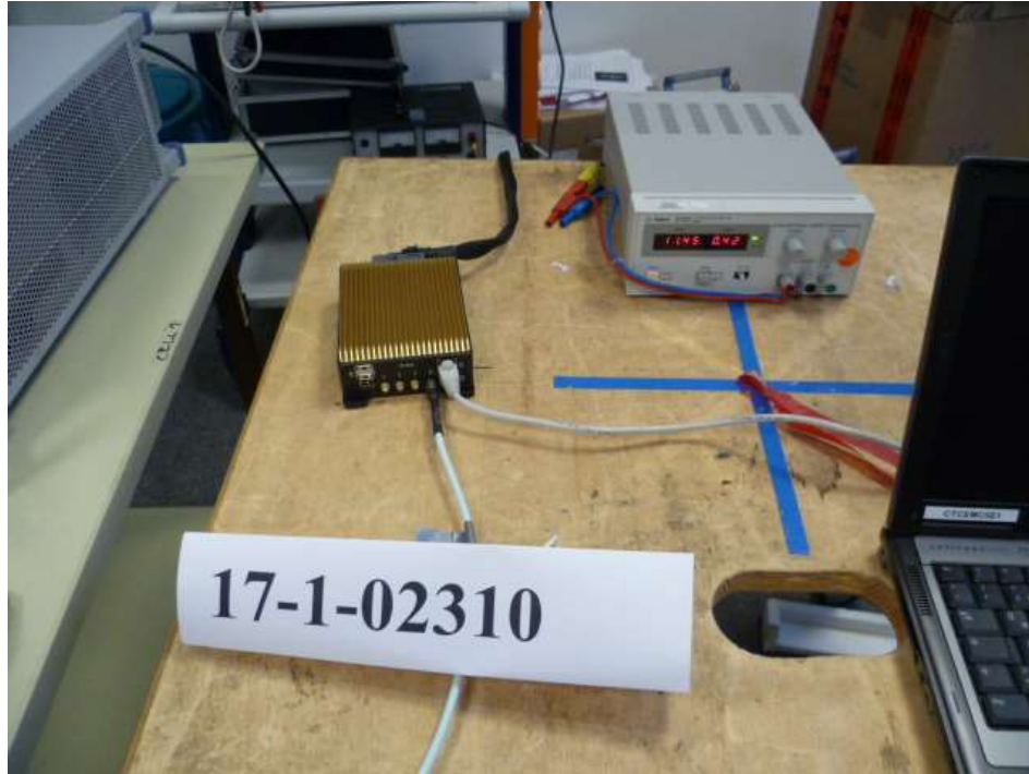
Figure 1: \mu CROS SL Conducted Measurement for Cellular Testing
