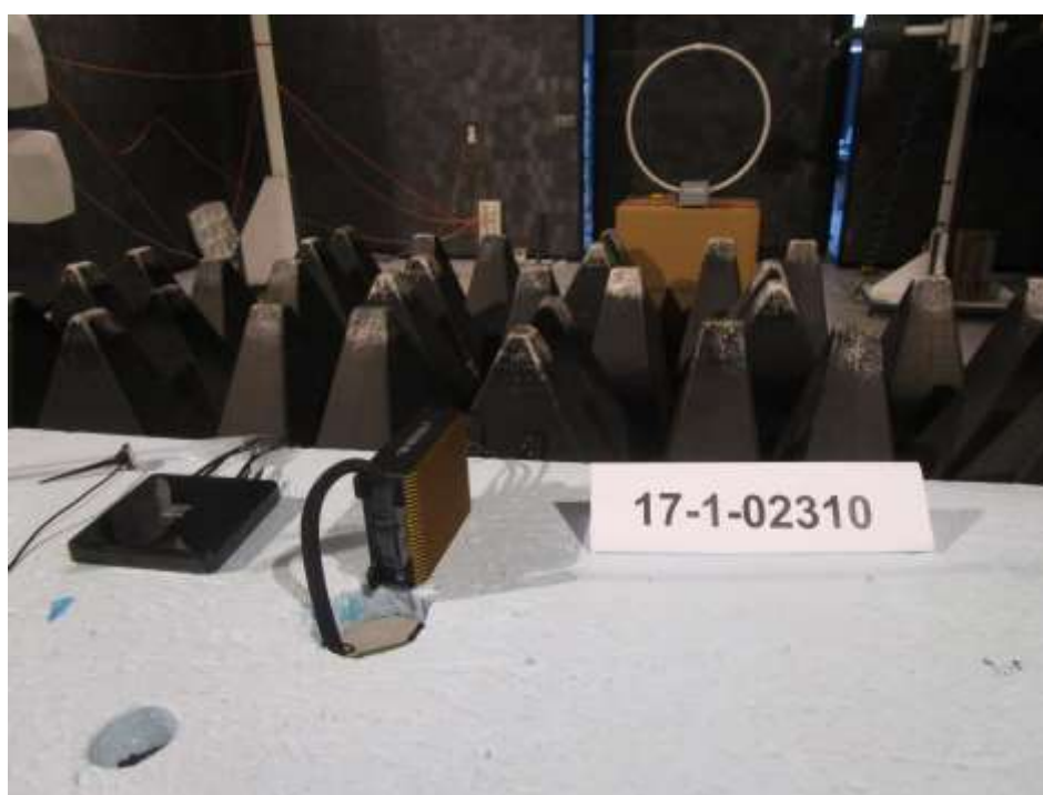
Figure 9: Overall View 9 KHz – 30 MHz EUT Standing
