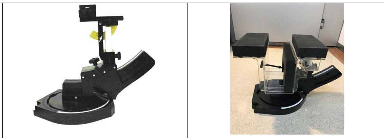
Device holder supplied by SPEAG
