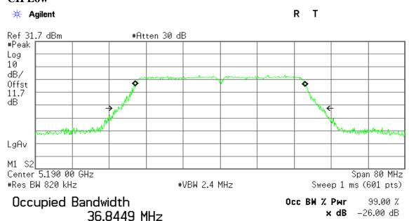
Transmit Freq Error -31.633 kHz x dB Bandwidth 43.849 MHz
