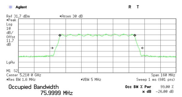
Transmit Freq Error 108.100 kHz x dB Bandwidth 83.886 MHz
