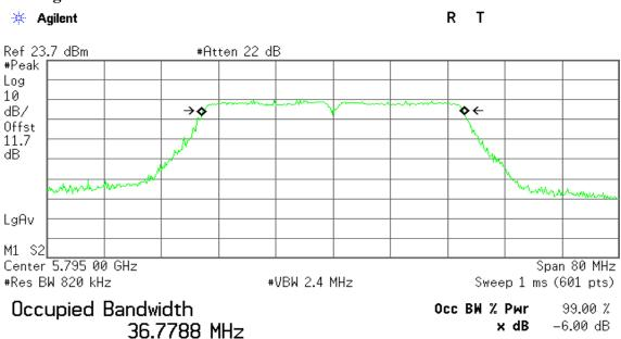
Transmit Freq Error 13.655 kHz x dB Bandwidth 36.451 MHz
