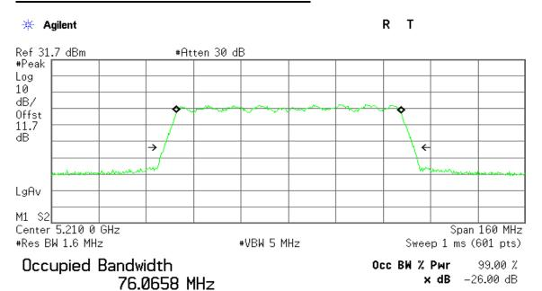
Transmit Freq Error 112.740 kHz x dB Bandwidth 84.391 MHz
