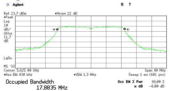
Transmit Freq Error 22.822 kHz x dB Bandwidth 17.753 MHz
