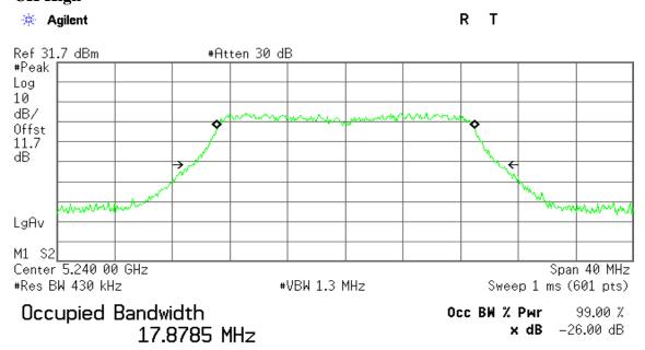
Transmit Freq Error 31.241 kHz x dB Bandwidth 21.280 MHz
