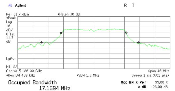
Transmit Freq Error -94.296 kHz x dB Bandwidth 23.521 MHz
