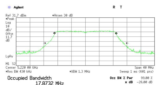
Transmit Freq Error 23.009 kHz x dB Bandwidth 21.758 MHz
