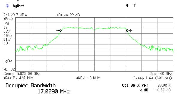
Transmit Freq Error -85.355 kHz x dB Bandwidth 16.521 MHz
