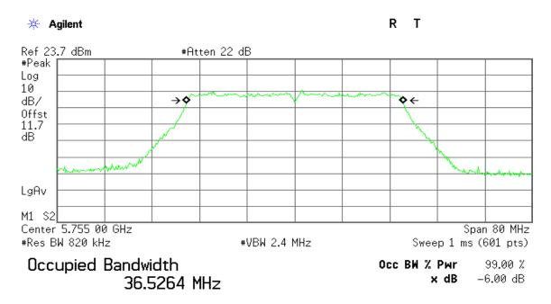
Transmit Freq Error 39.909 kHz x dB Bandwidth 36.104 MHz
