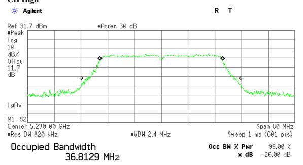
Transmit Freq Error -35.020 kHz x dB Bandwidth 43.874 MHz
