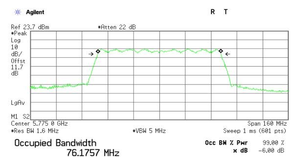
Transmit Freq Error -35.039 kHz x dB Bandwidth 76.596 MHz
