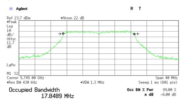
Transmit Freq Error 23.670 kHz x dB Bandwidth 17.691 MHz
