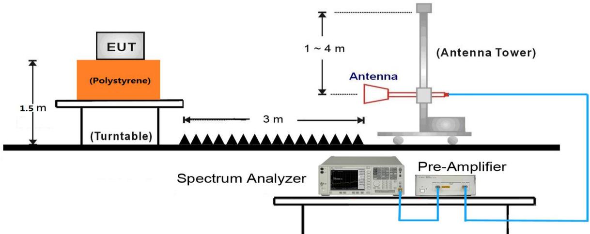
Above 40GHz Test Setup:
