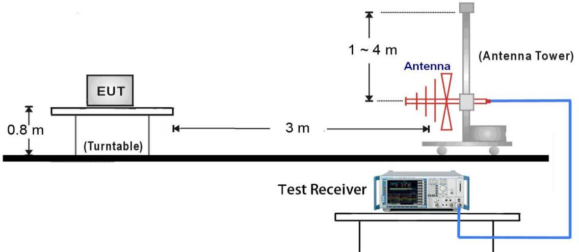
1GHz ~ 40GHz Test Setup:
