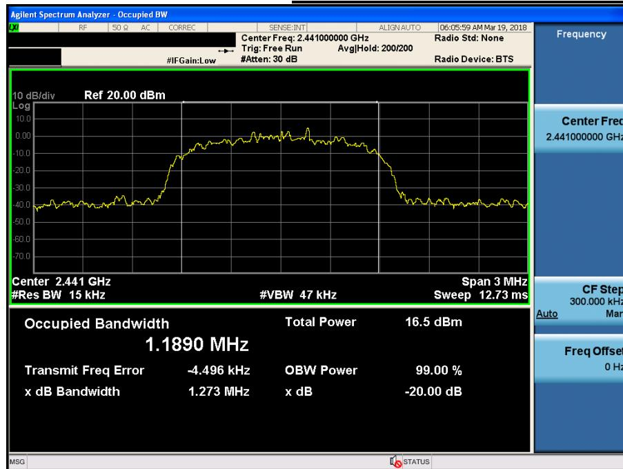
**20 dB Bandwidth****Highest Channel & Modulation : 8DPSK**
