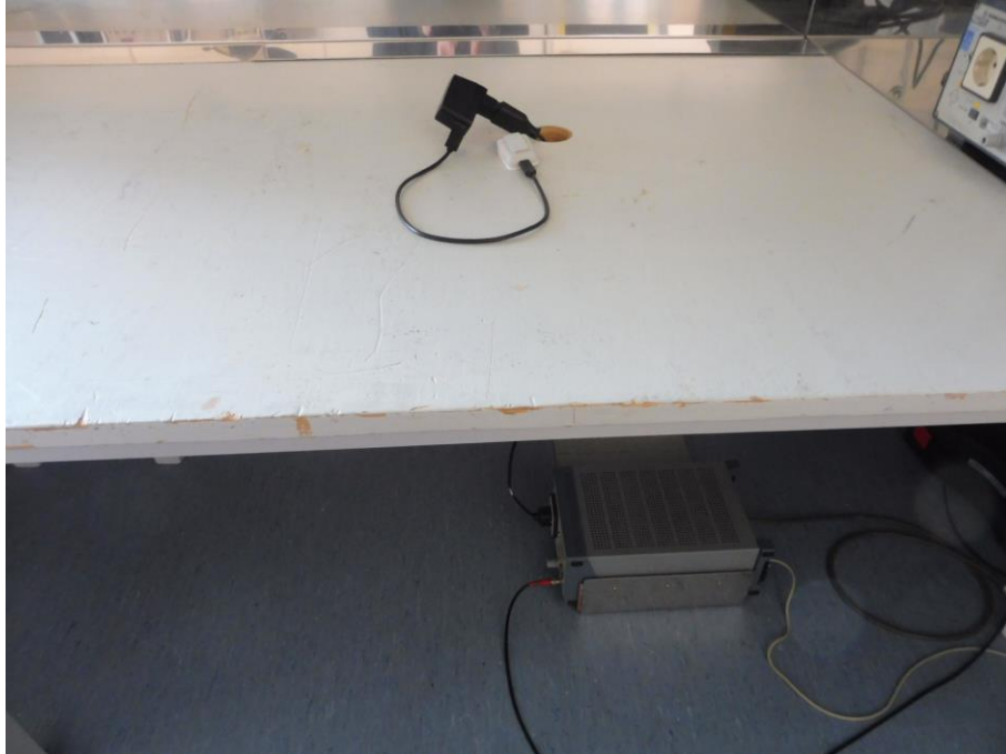
Photo 9: Conducted AC Emissions
