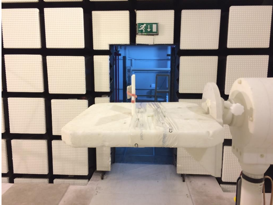
Photo 3: RSE set-up (>1GHz)
