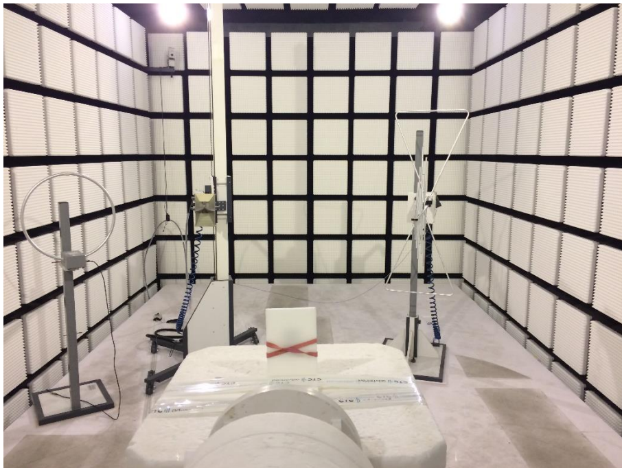
Photo 2: RSE set-up (>1GHz)
