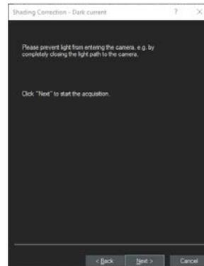
4. After the dark current image calibration select all objectives. Immersion objectives are calibrated in the same wizard. However the calibration wizard will calibrate all dry objectives first and subsequently select the immersion medium objective(s).
