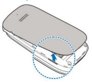
Place the nano-SIM card with the chip facing downwards and the cut corner oriented as shown and slide the nano-SIM card into the card holder.
