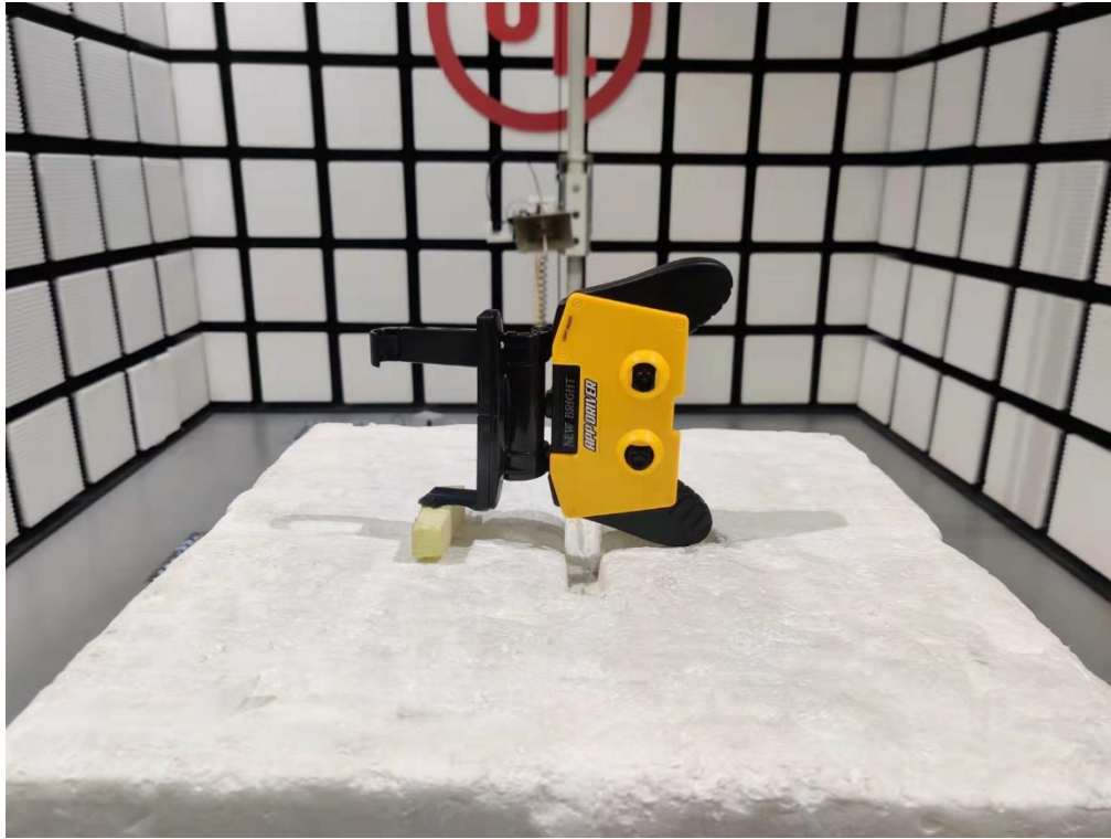
Radiated Disturbance Setup (Above 1 GHz – Z axis)
