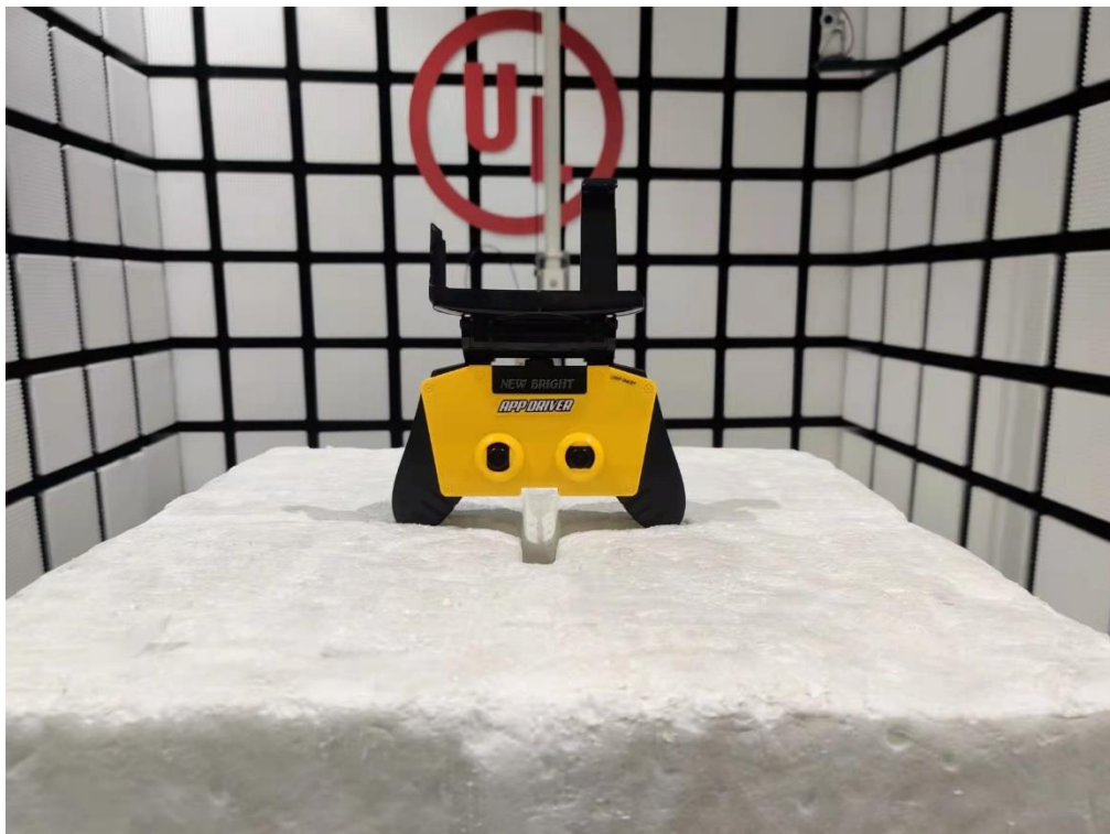
Radiated Disturbance Setup (Above 1 GHz – Y axis)
