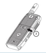
**3** Slide the battery latch into lock position.
