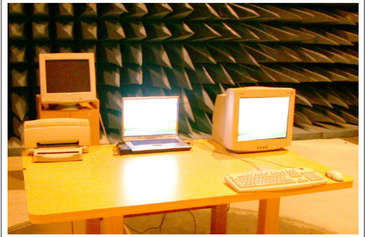
The Front View of Highest Radiated Set-up For EUT
