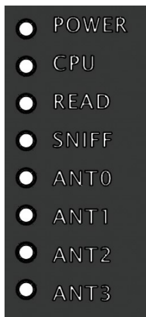
Figure 7 – ALR-F800 Front Panel Reader Diagnostic LEDs
