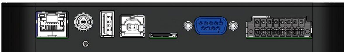
Figure 8 – Power, RS-232, USB, SDCard and LAN Connections
