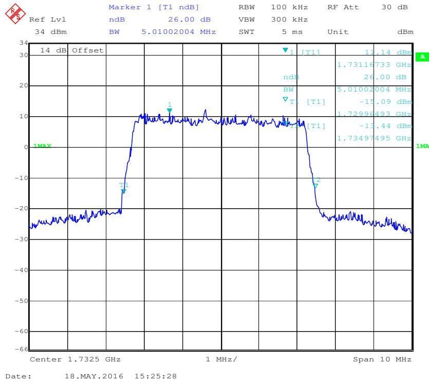
**16-QAM (5.0 MHz) - 99% Occupied Bandwidth, Middle channel**
