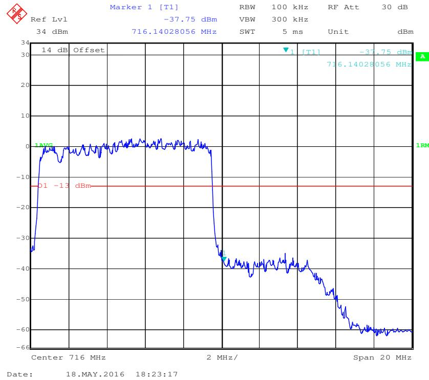
**16-QAM (10 MHz, FULL RB) - Left Band Edge**
