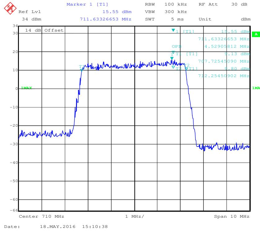
**16-QAM (5.0 MHz) - 26 dB Bandwidth, Middle channel**
