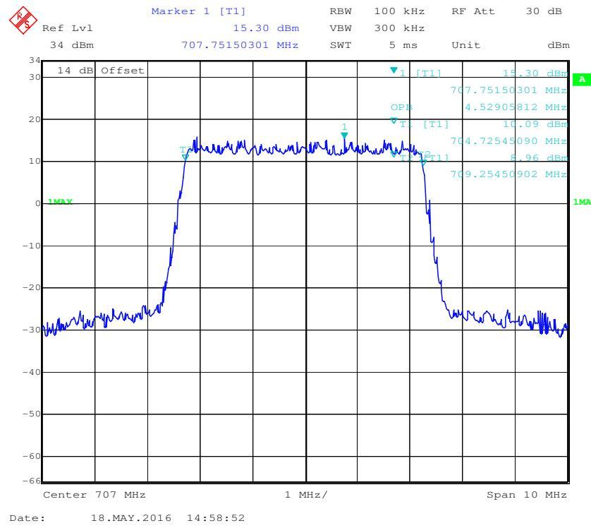
**QPSK (5.0 MHz) -26 dB Bandwidth, Middle channel**
