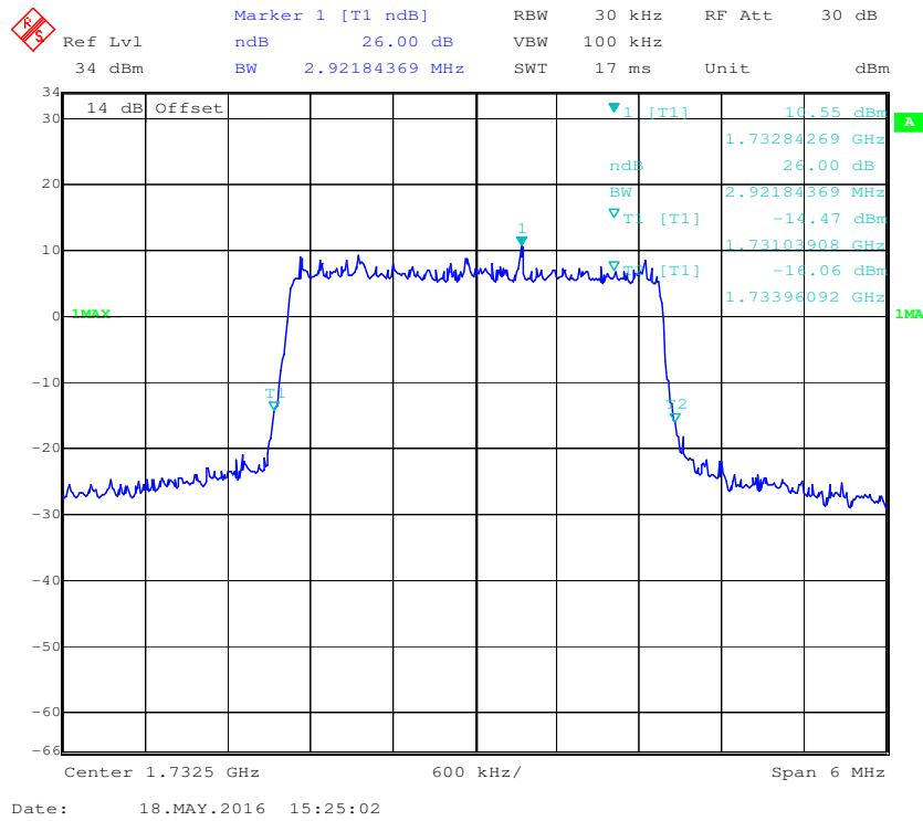
**16-QAM (3.0 MHz) - 99% Occupied Bandwidth, Middle channel**
