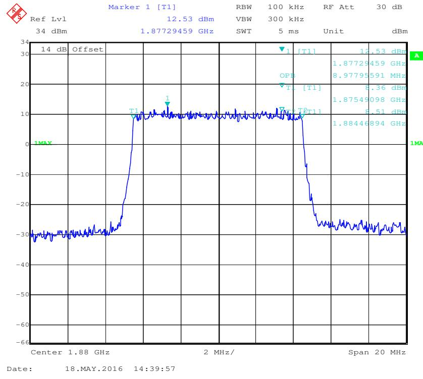
**QPSK (10.0 MHz) -26 dB Bandwidth, Middle channel**
