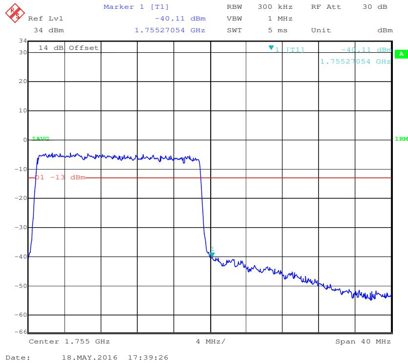
**Band 12:****QPSK (1.4 MHz, FULL RB) - Left Band Edge**
