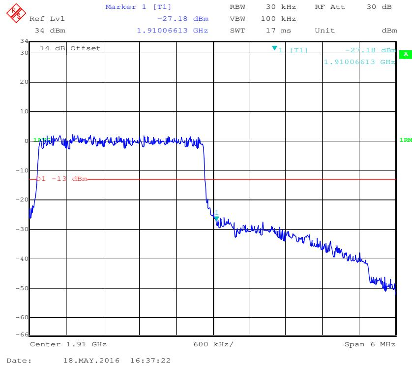
**16-QAM (3.0 MHz, FULL RB) - Left Band Edge**
