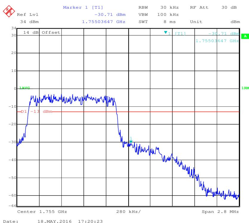
**16-QAM (1.4 MHz, FULL RB) - Left Band Edge**
