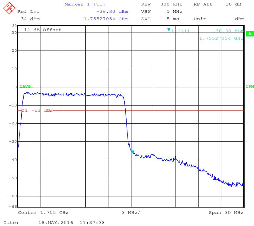
**QPSK (20.0 MHz, FULL RB) - Left Band Edge**
