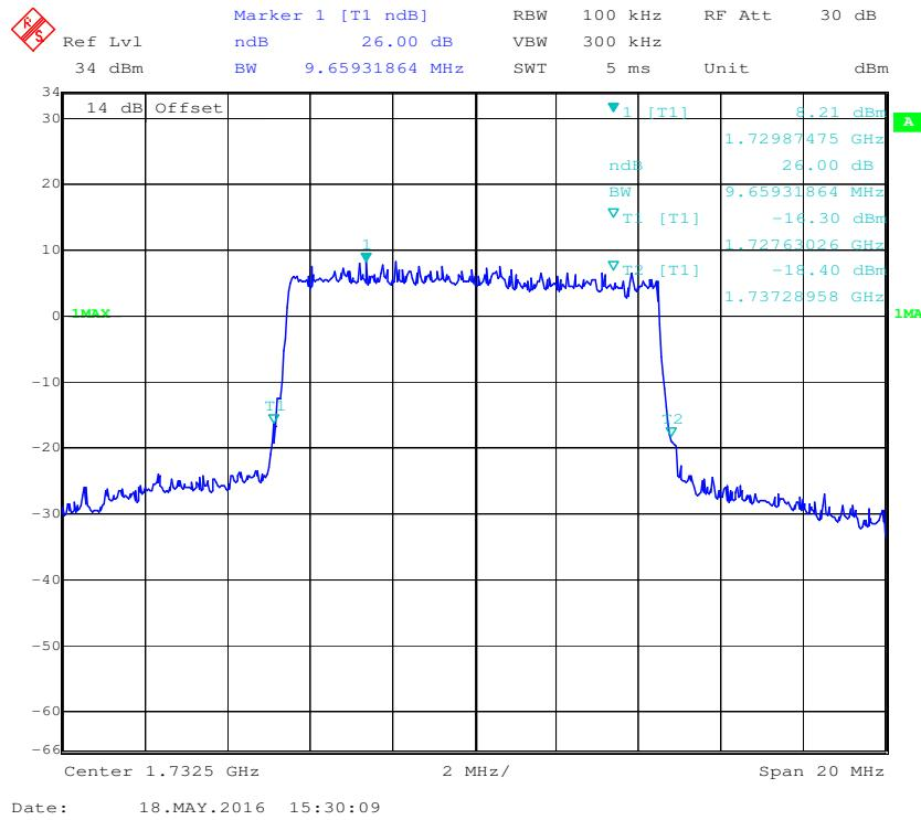
**QPSK (15.0 MHz) - 99% Occupied Bandwidth, Middle channel**
