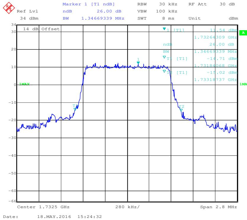
**16-QAM (1.4 MHz) -99% Occupied Bandwidth Middle channel**
