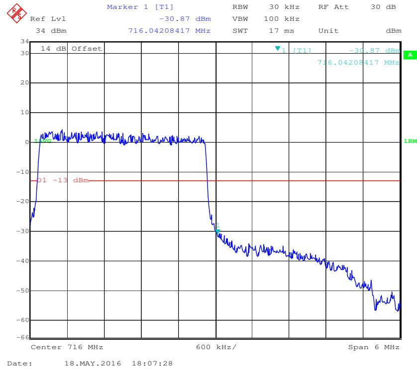
**16-QAM (3.0 MHz, FULL RB) - Left Band Edge**
