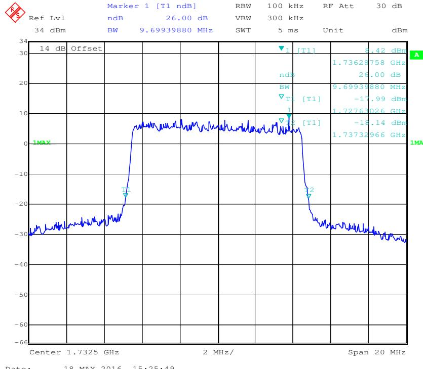
**16-QAM (10.0 MHz) - 99% Occupied Bandwidth, Middle channel**
