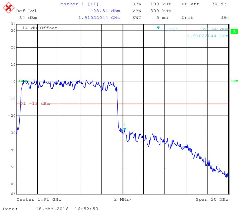
**QPSK (15.0 MHz, FULL RB) - Left Band Edge**
