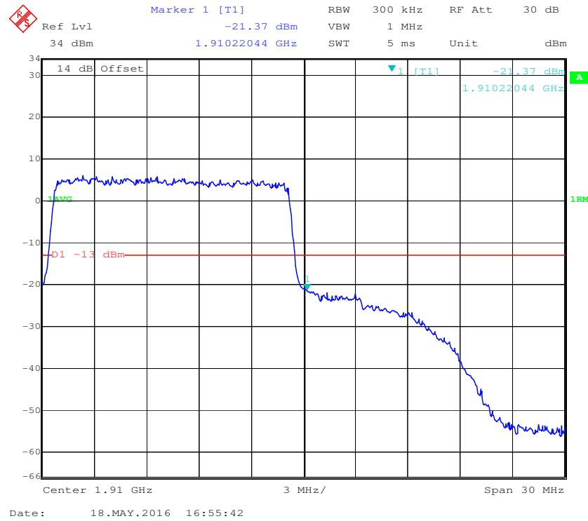
**16-QAM (15.0 MHz, FULL RB) - Left Band Edge**
