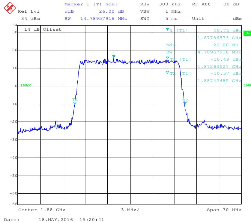
**QPSK (20.0 MHz) - 99% Occupied Bandwidth, Middle channel**
