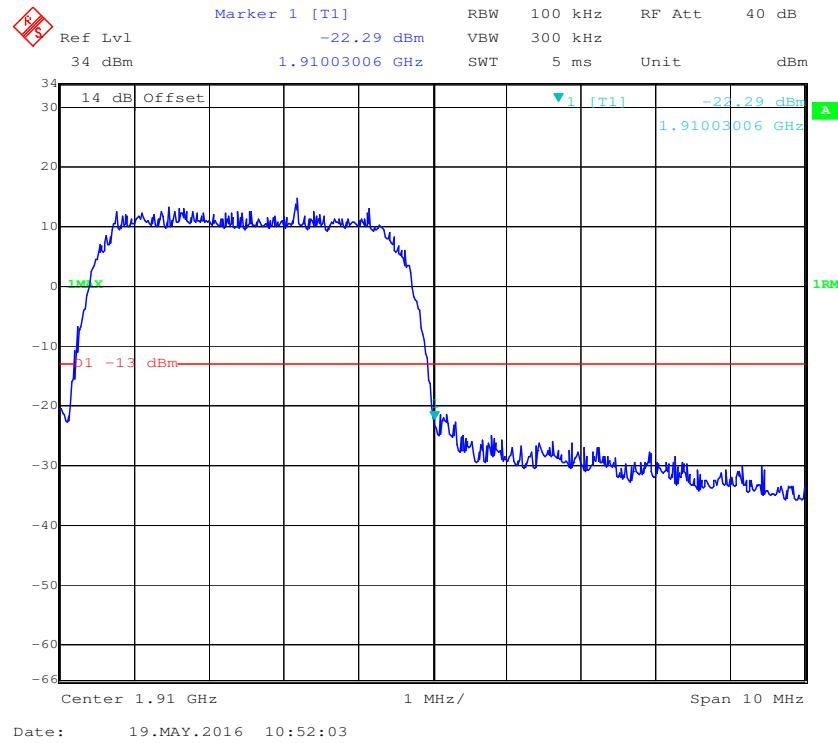
**Band 2:****QPSK (1.4 MHz, FULL RB) - Left Band Edge**
