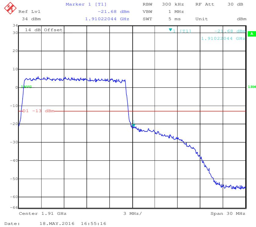
**QPSK (20.0 MHz, FULL RB) - Left Band Edge**
