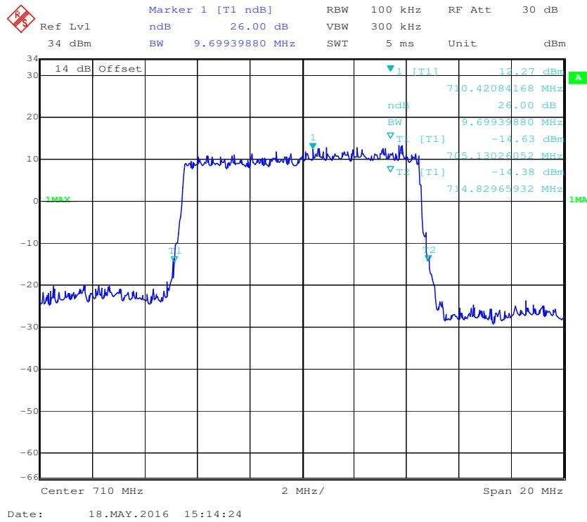
**16-QAM (10.0 MHz) - 99% Occupied Bandwidth, Middle channel**
