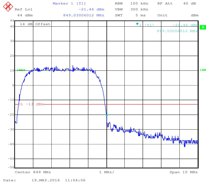
**Cellular Band, Left Band Edge for HSDPA (16QAM) Mode**
