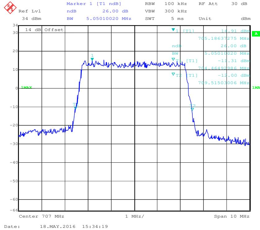
**QPSK (10.0 MHz) - 99% Occupied Bandwidth, Middle channel**
