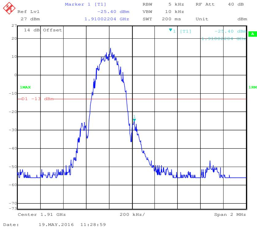
**PCS Band, Left Band Edge for RMC (BPSK) Mode**
