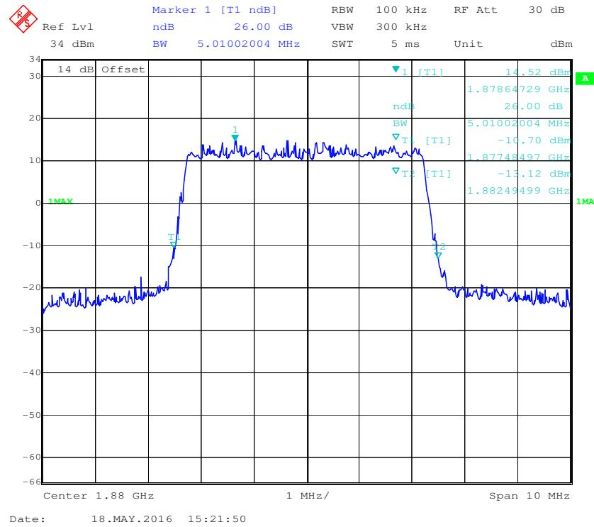
**QPSK (10.0 MHz) - 99% Occupied Bandwidth, Middle channel**
