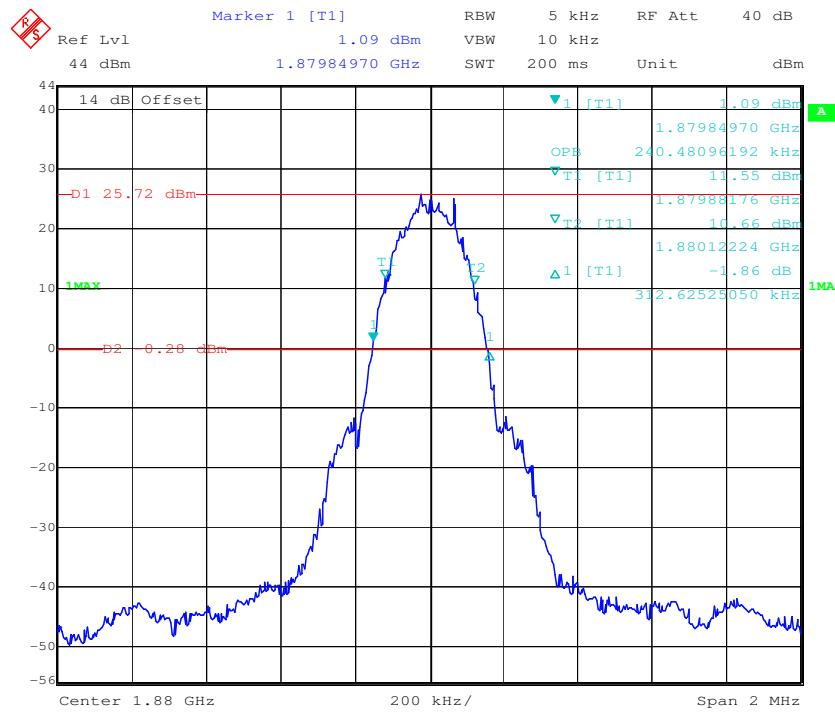
**99%&26 dB Occupied Bandwidth for EGPRS Mode**
