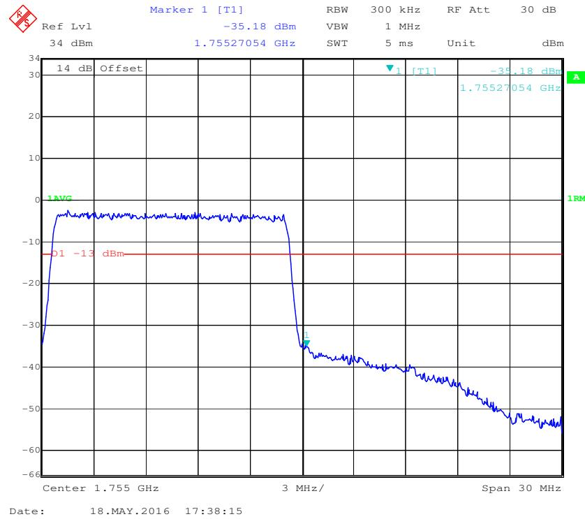
**16-QAM (15.0 MHz, FULL RB) - Left Band Edge**
