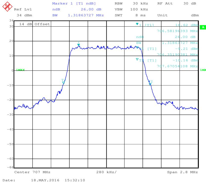
**16-QAM (1.4 MHz) - 99% Occupied Bandwidth, Middle channel**
