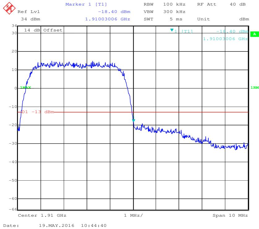
**PCS Band, Left Band Edge for HSDPA (16QAM) Mode**
