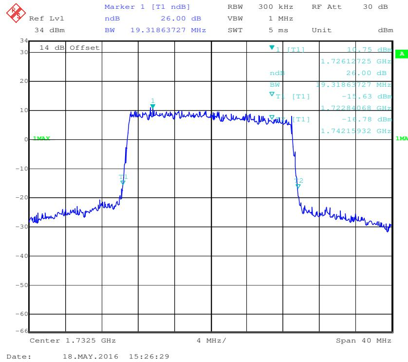
**16-QAM (20.0 MHz) - 99% Occupied Bandwidth, Middle channel**
