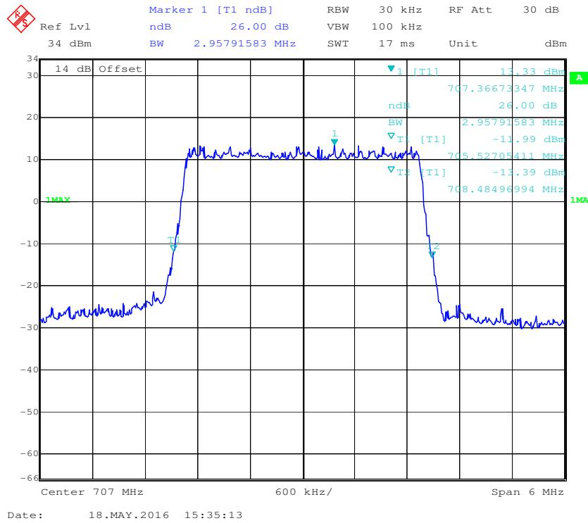
**QPSK (5.0 MHz) -99% Occupied Bandwidth, Middle channel**
