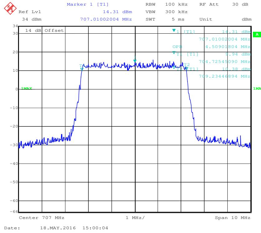
**16-QAM (5.0 MHz) -26 dB Bandwidth, Middle channel**
