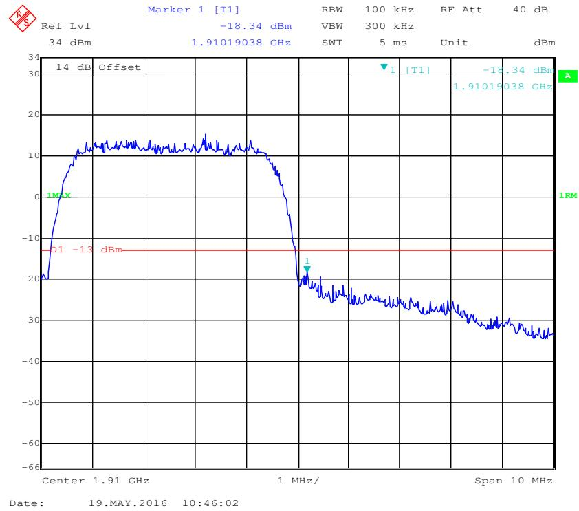
**PCS Band, Left Band Edge for HSUPA (BPSK) Mode**
