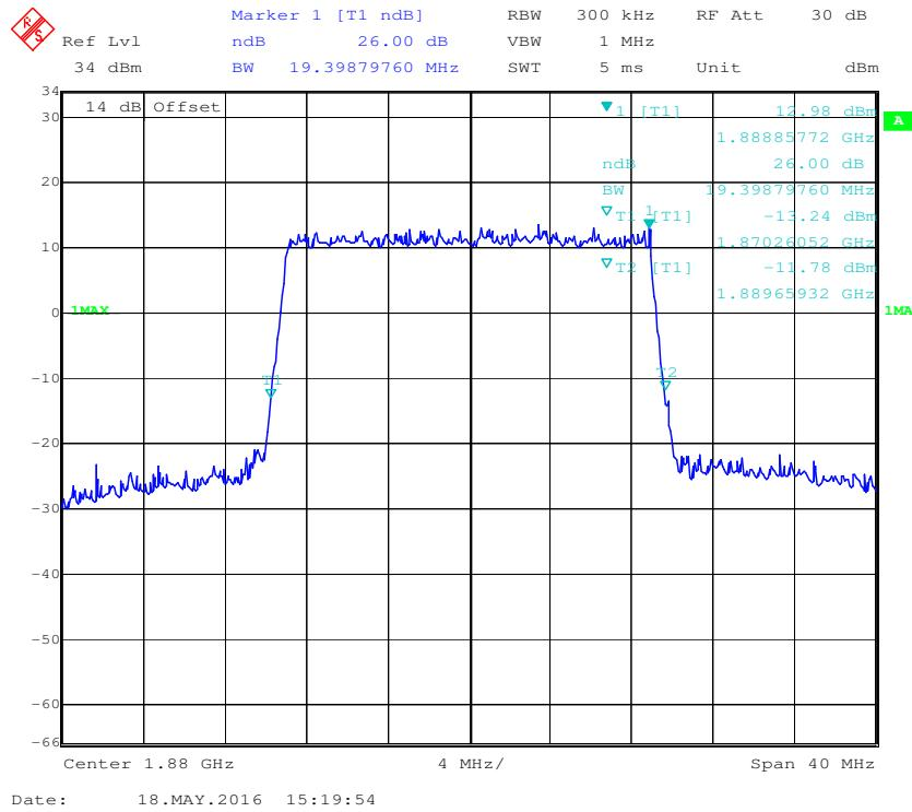
**16-QAM (20.0 MHz) - 99% Occupied Bandwidth, Middle channel**
