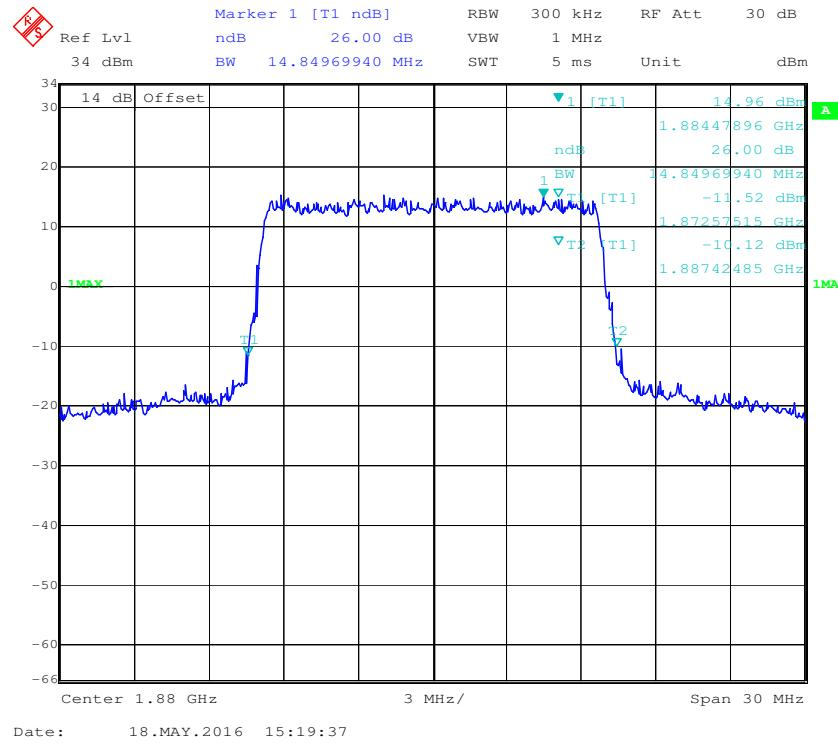
**16-QAM (15.0 MHz) - 99% Occupied Bandwidth, Middle channel**
