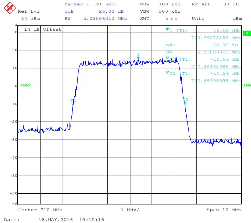
**QPSK (10.0 MHz) - 99% Occupied Bandwidth, Middle channel**
