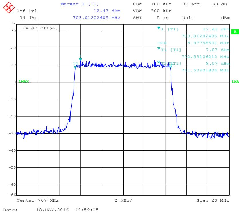
**QPSK (10.0 MHz) - 26 dB Bandwidth, Middle channel**
