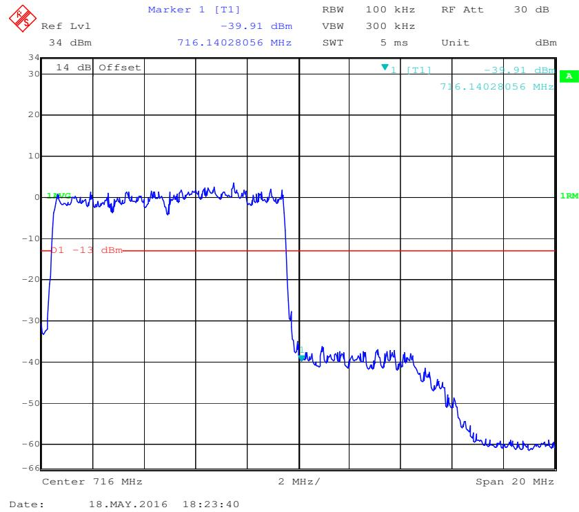
**Band 17:****QPSK (5 MHz, FULL RB) - Left Band Edge**
