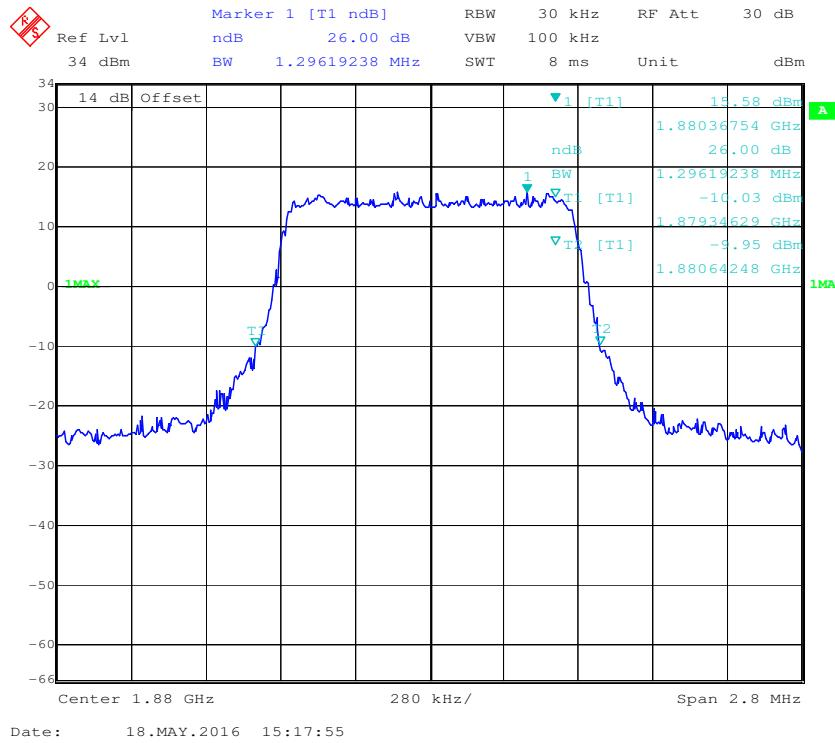
**16-QAM (1.4 MHz) -99% Occupied Bandwidth Middle channel**
