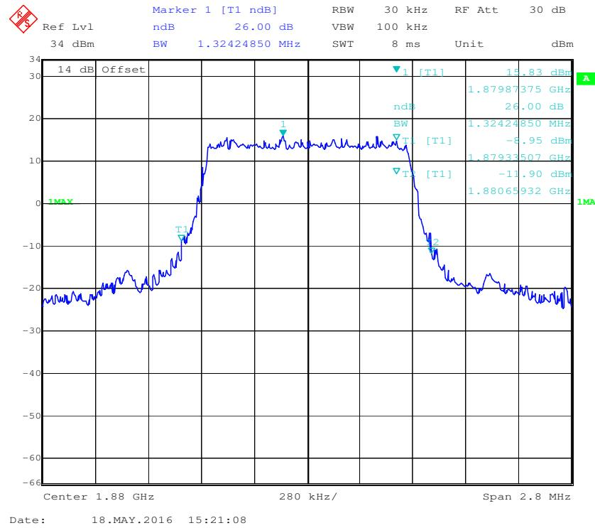
**QPSK (3.0 MHz) - 99% Occupied Bandwidth, Middle channel**
