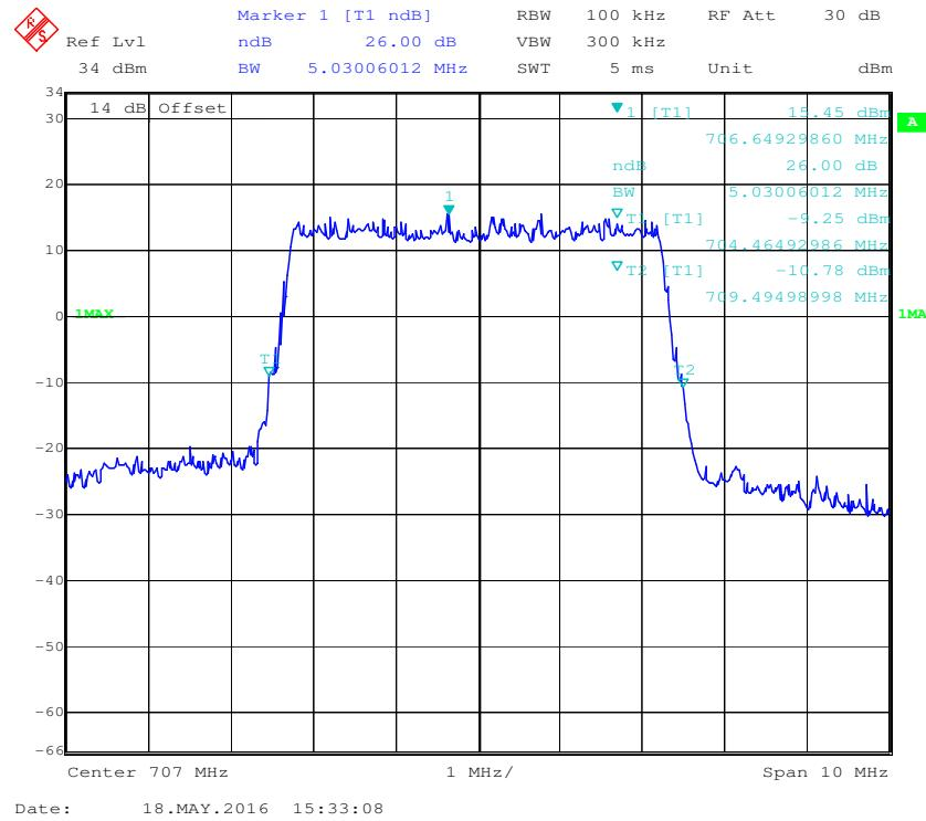
**16-QAM (5.0 MHz) -99% Occupied Bandwidth, Middle channel**
