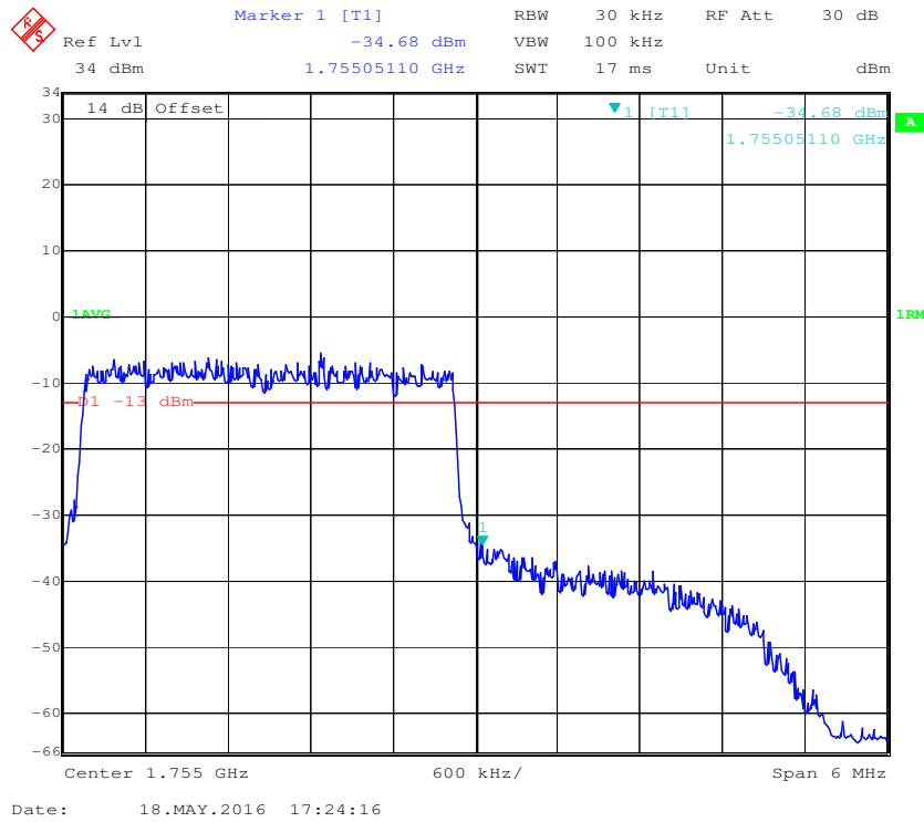
**16-QAM (3.0 MHz, FULL RB) - Left Band Edge**
