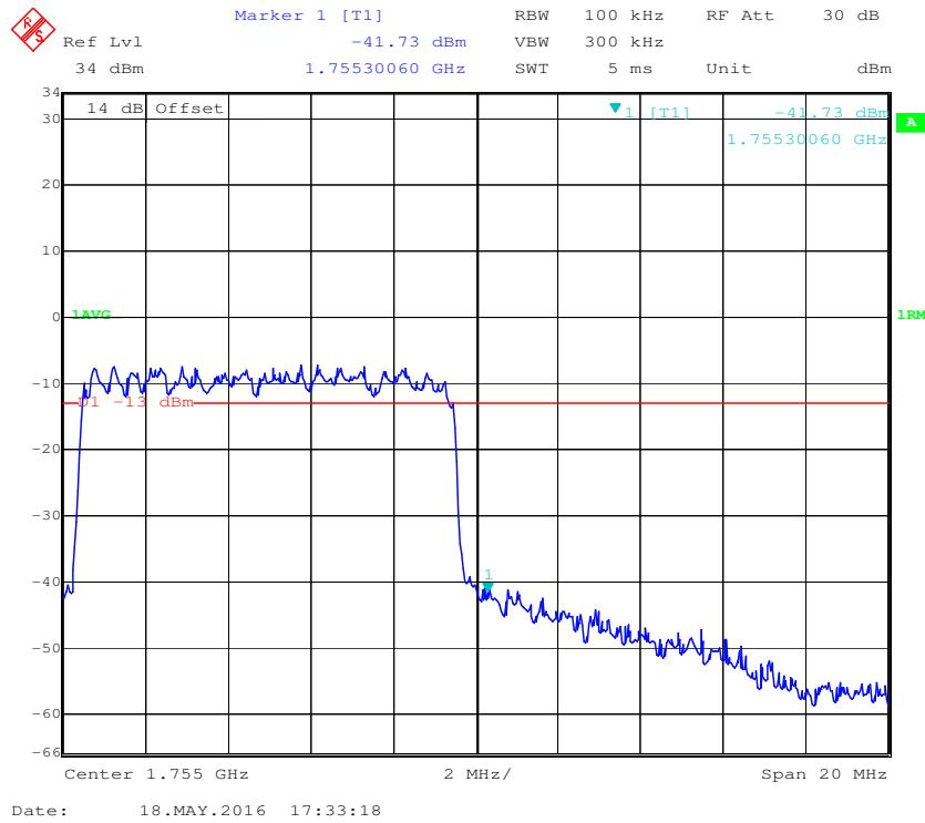
**QPSK (15.0 MHz, FULL RB) - Left Band Edge**
