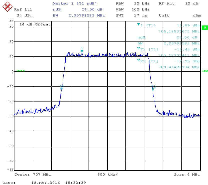
**16-QAM (3.0 MHz) - 99% Occupied Bandwidth, Middle channel**
