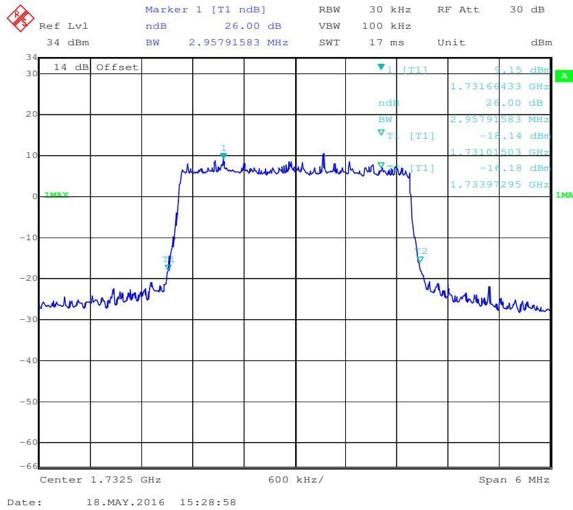
**QPSK (5.0 MHz) - 99% Occupied Bandwidth, Middle channel**
