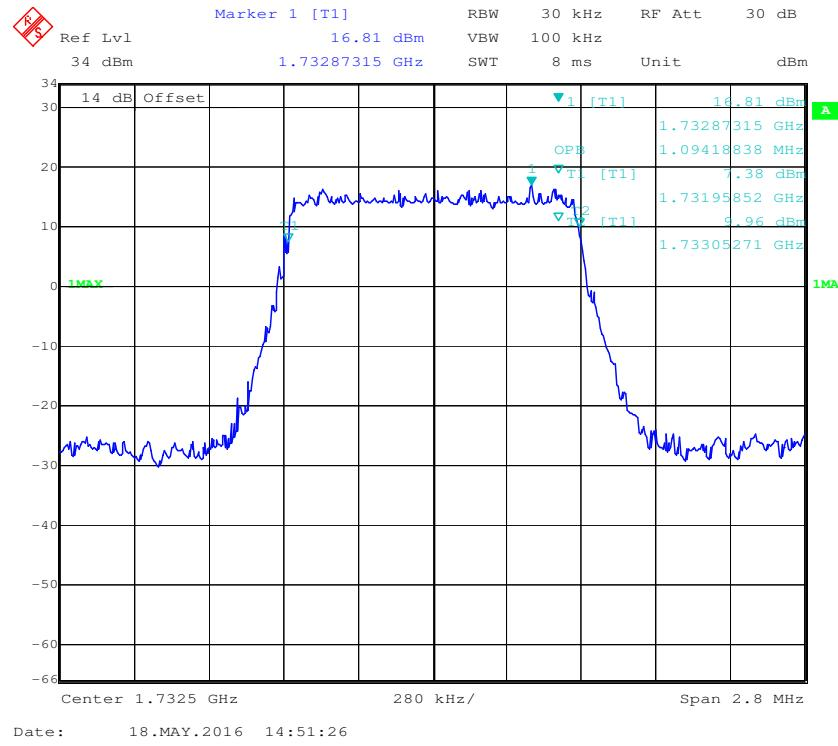
**16-QAM (1.4 MHz) -26 dB Bandwidth Middle channel**
