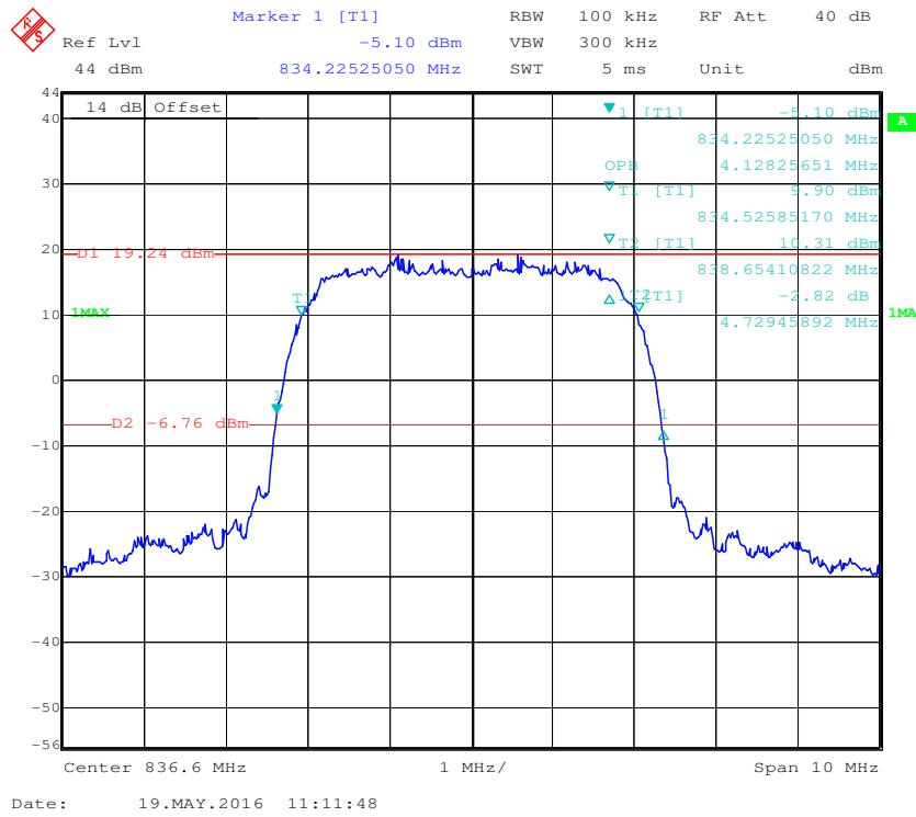
**99%&26 dB Occupied Bandwidth for HSDPA (16QAM) Mode**
