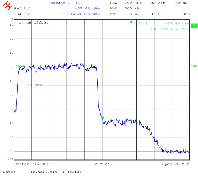
**16-QAM (10 MHz, FULL RB) - Left Band Edge**
