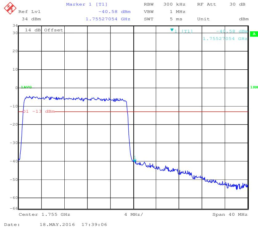
**16-QAM (20.0 MHz, FULL RB) - Left Band Edge**
