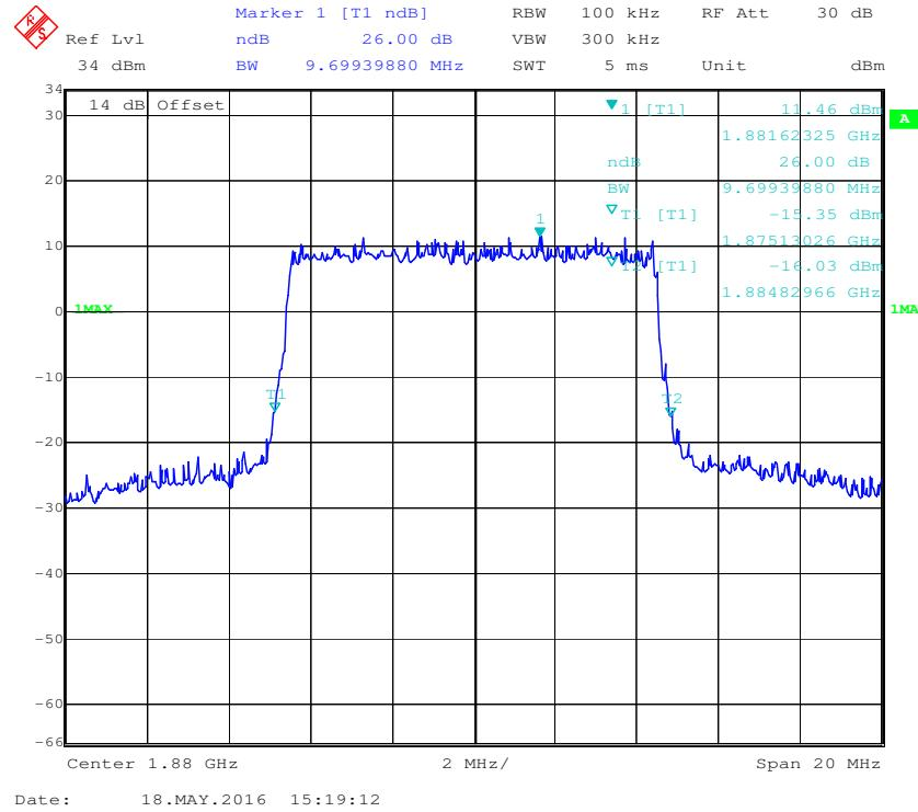
**16-QAM (10.0 MHz) - 99% Occupied Bandwidth, Middle channel**
