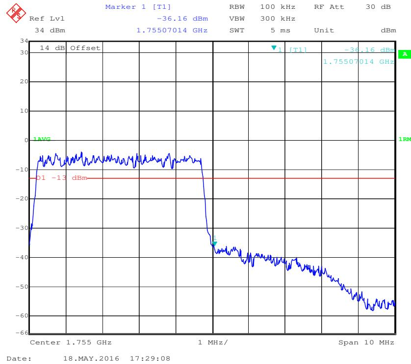
**QPSK (10.0 MHz, FULL RB) - Left Band Edge**
