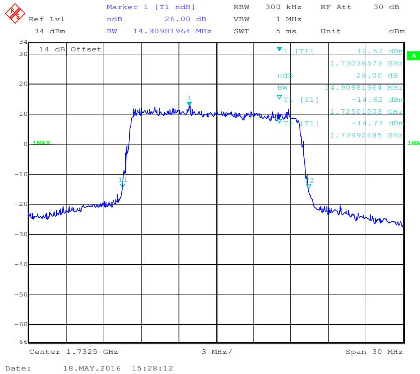
**QPSK (20.0 MHz) - 99% Occupied Bandwidth, Middle channel**
