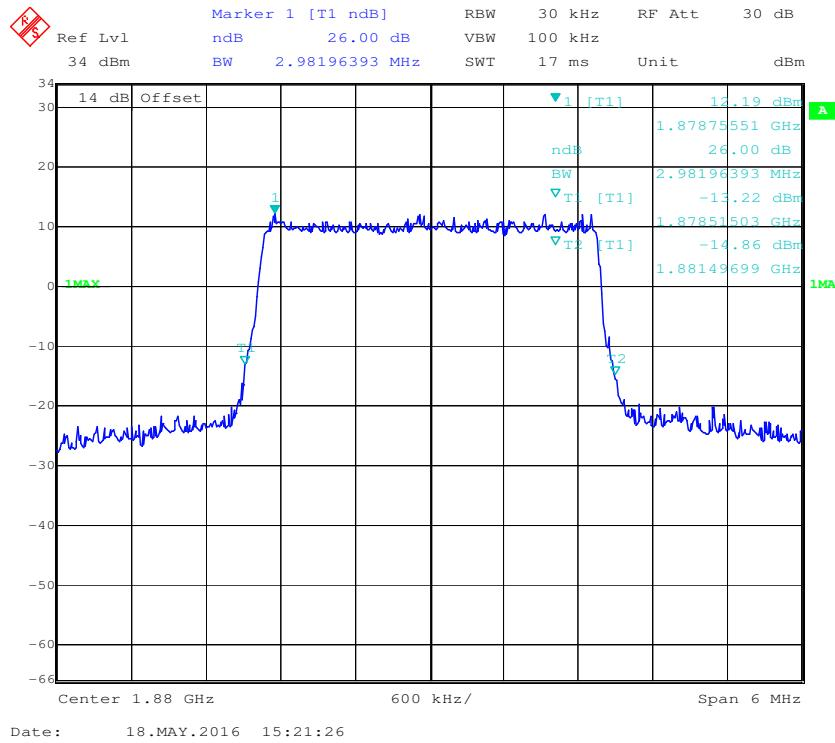
**QPSK (5.0 MHz) - 99% Occupied Bandwidth, Middle channel**
