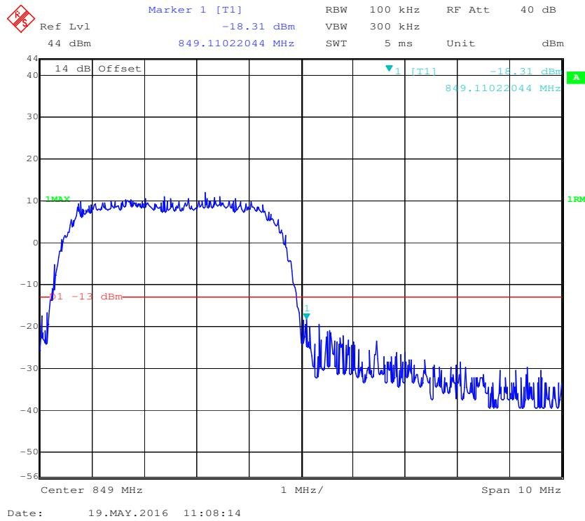
**Cellular Band, Left Band Edge for HSUPA (BPSK) Mode**
