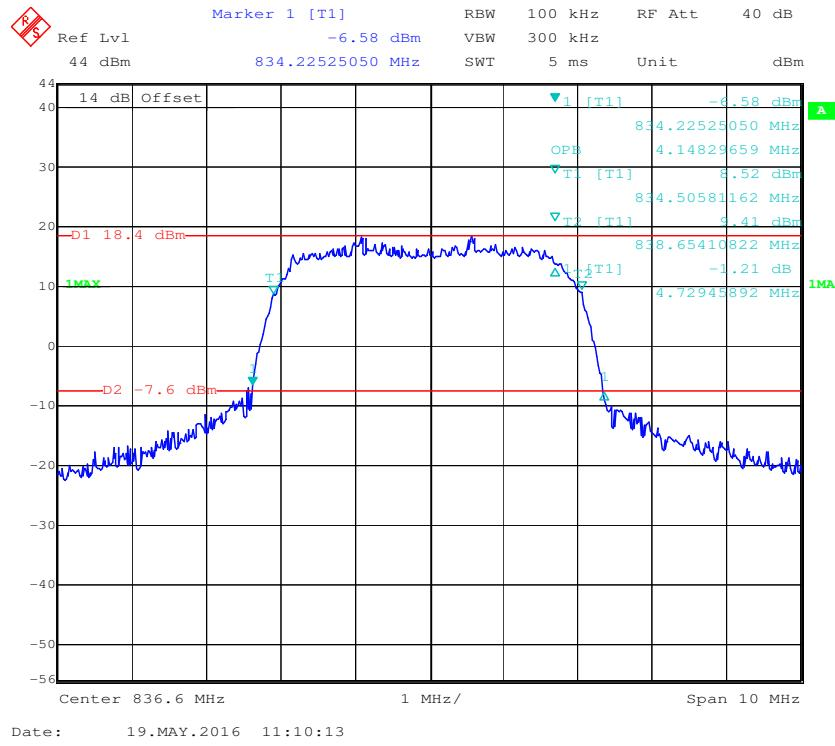
**PCS Band (Part 24E)****99%&26 dB Occupied Bandwidth for GSM (GMSK) Mode**
