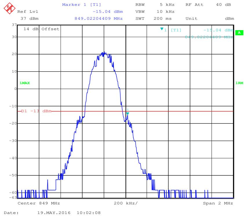
**Cellular Band, Left Band Edge for EGPRS Mode**
