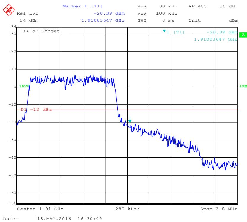
**16-QAM (1.4 MHz, FULL RB) - Left Band Edge**
