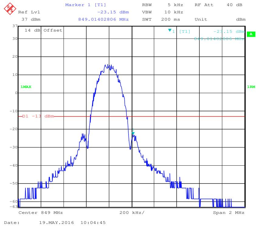
**Cellular Band, Left Band Edge for RMC (BPSK) Mode**
