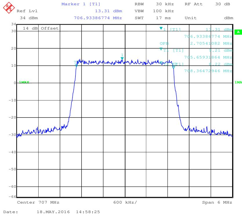
**QPSK (3.0 MHz) - 26 dB Bandwidth, Middle channel**
