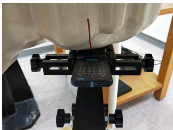
Fig.5 Left Head Section / Cheek-Touch Position
