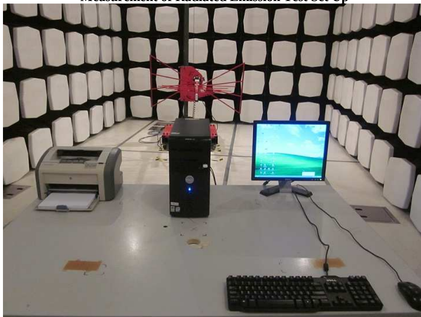
Measurement of Radiated Emission Test Set Up
