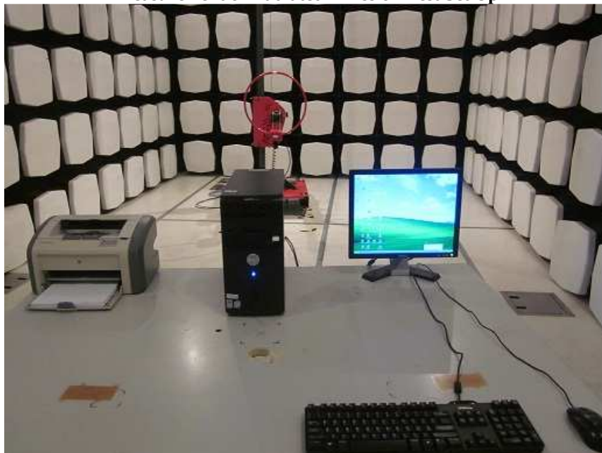
Measurement of Radiated Emission Test Set Up
