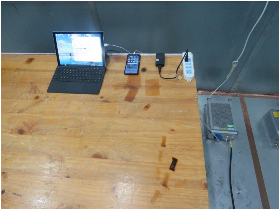
Picture 1: Conducted Emissions Test Setup
