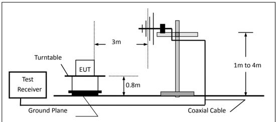
(c) For radiated emissions above 1000MHz
