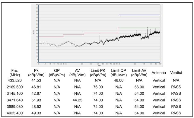
(433.92 MHz, Antenna Vertical, 30 MHz to 5 GHz)
