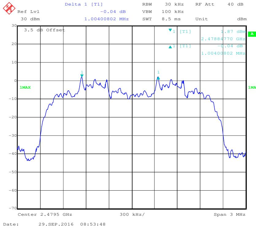
**EDR (8DPSK): Low Channel**
