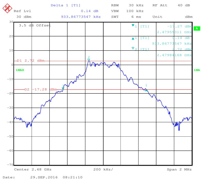
**EDR ( $\pi/4$ -DQPSK): Low Channel**
