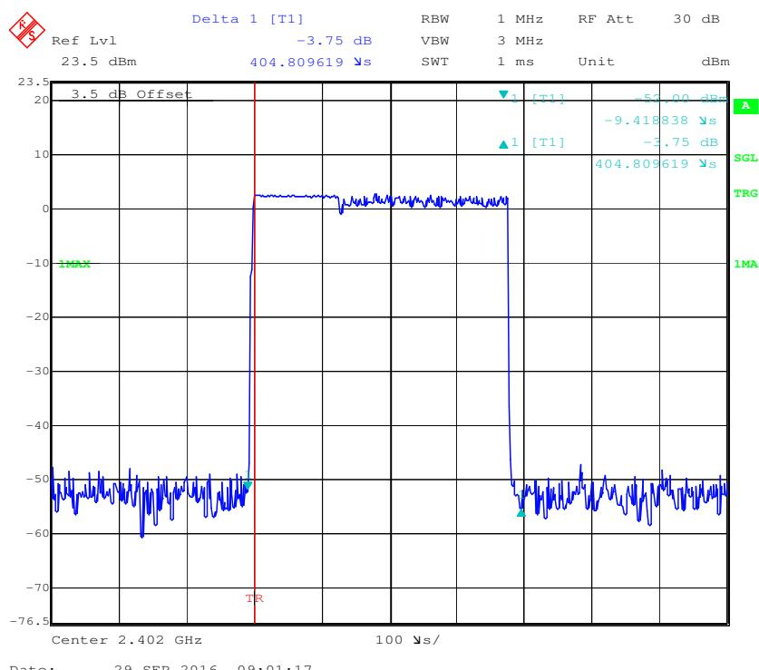
**Pulse time, Middle Channel, 2DH1**
