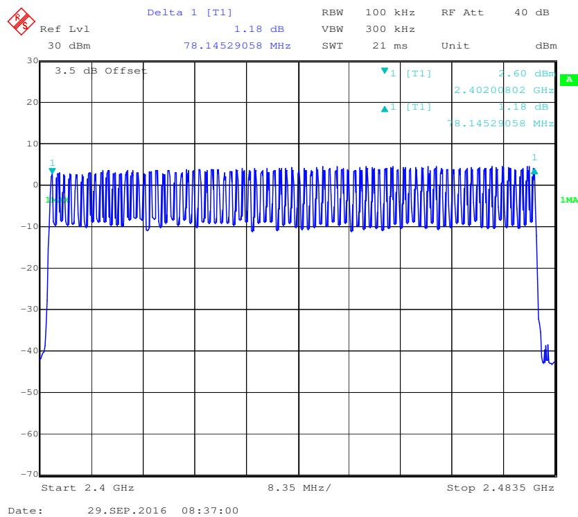
**EDR ( $\pi/4$ -DQPSK): Number of Hopping Channels**
