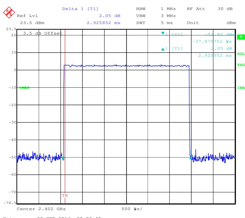
**Pulse time, Middle Channel, 2DH5**
