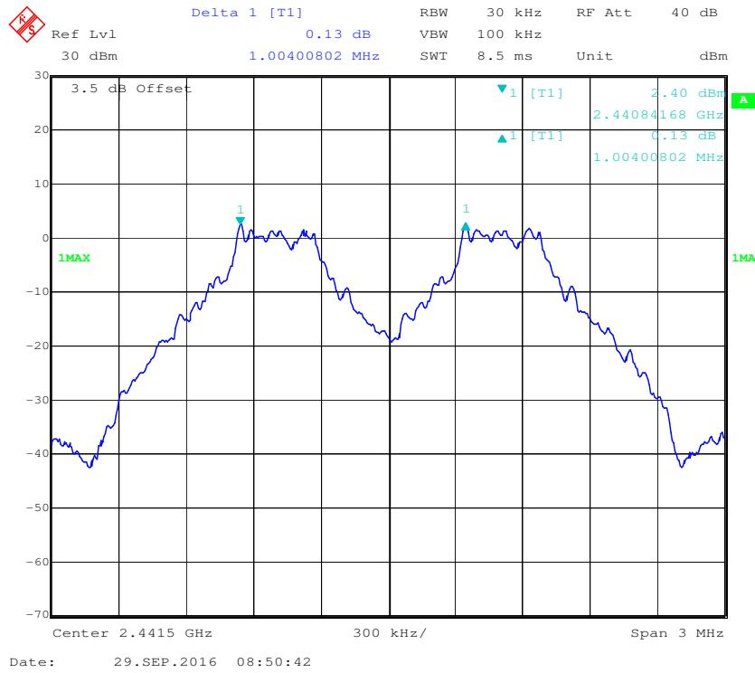
**BDR (GFSK): High Channel**
