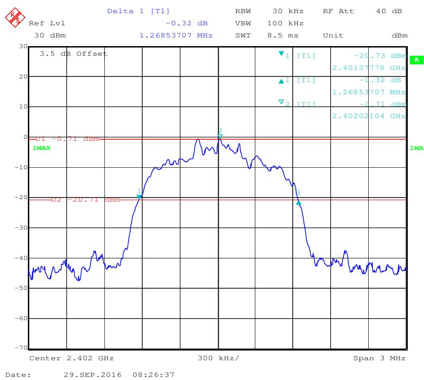
**EDR (8DPSK): Middle Channel**
