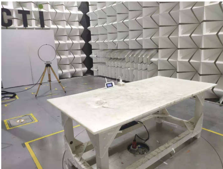
Radiated spurious emission Test Setup-1(Below 30MHz)
