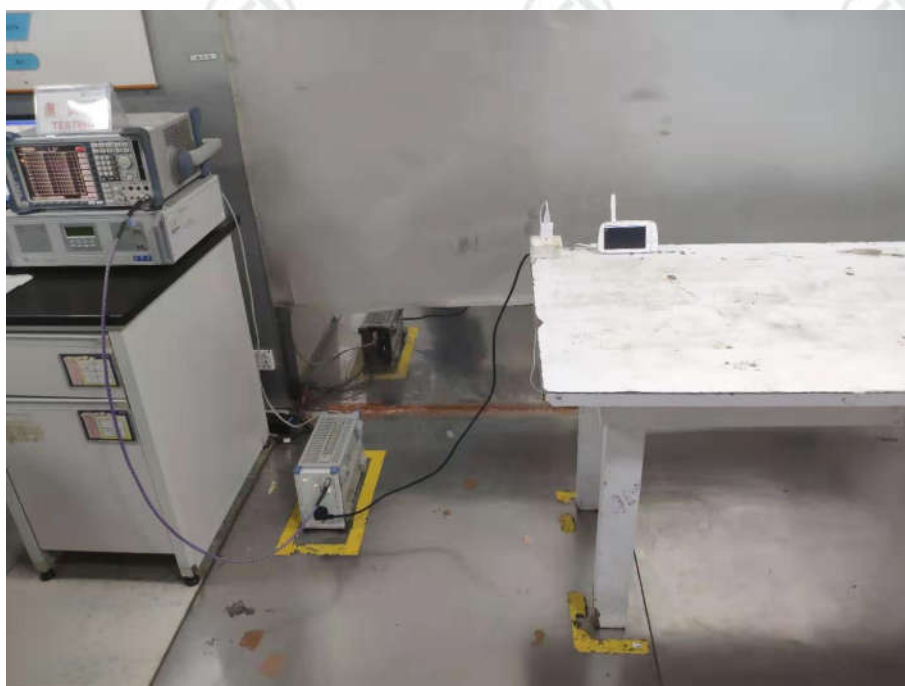
Conducted Emissions Test Setup
