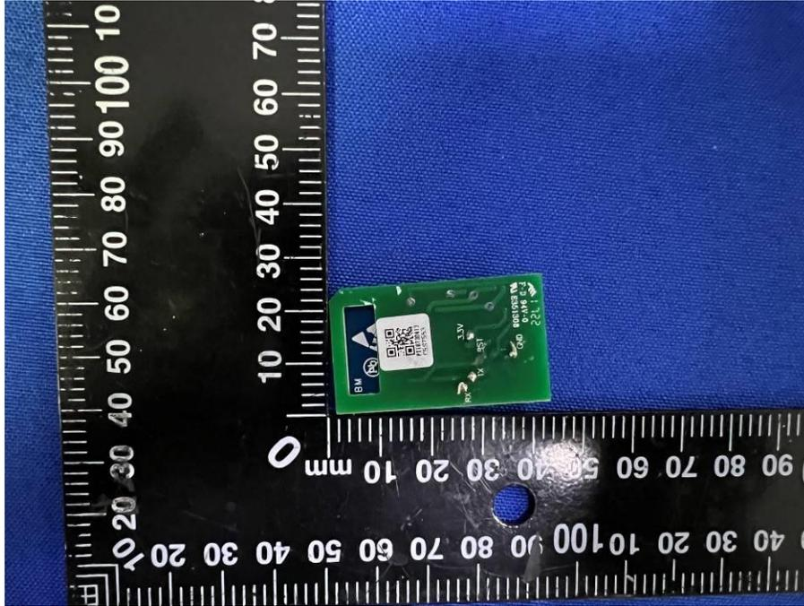
View of RF Module and Antenna location-1
