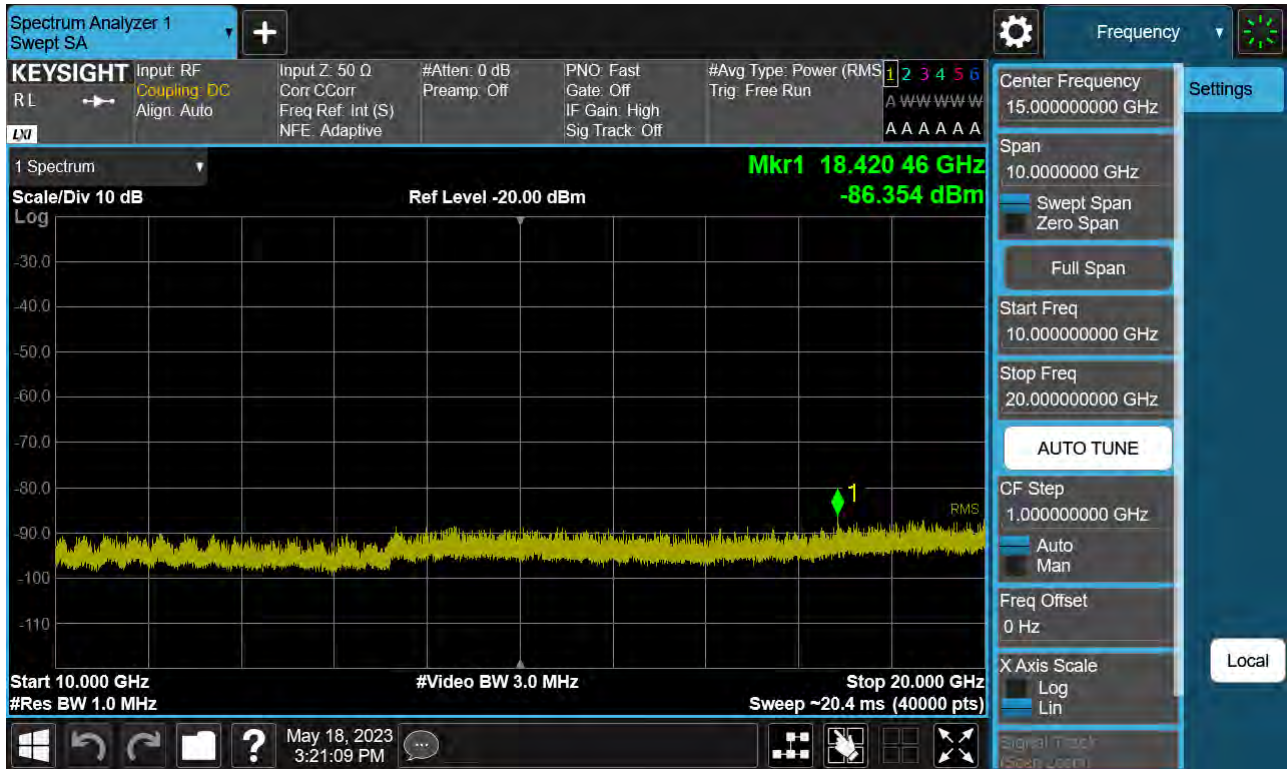
Sub6 n66. Conducted Spurious Plot_2 (349000ch_10 MHz_BPSK_ RB 1_1)
