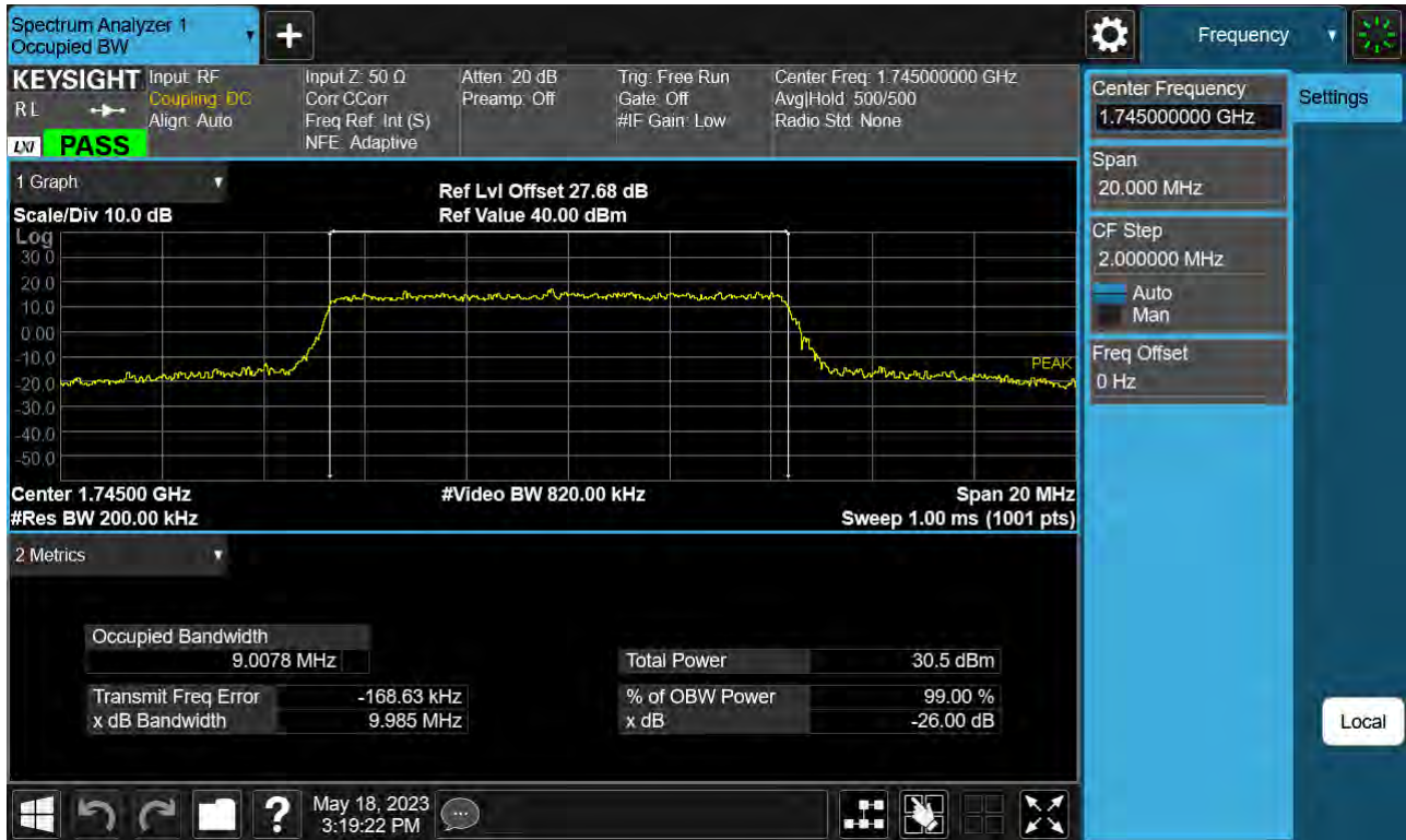
Sub6 n66. Occupied Bandwidth Plot (10 M BW Ch.349000 16QAM Full RB)
