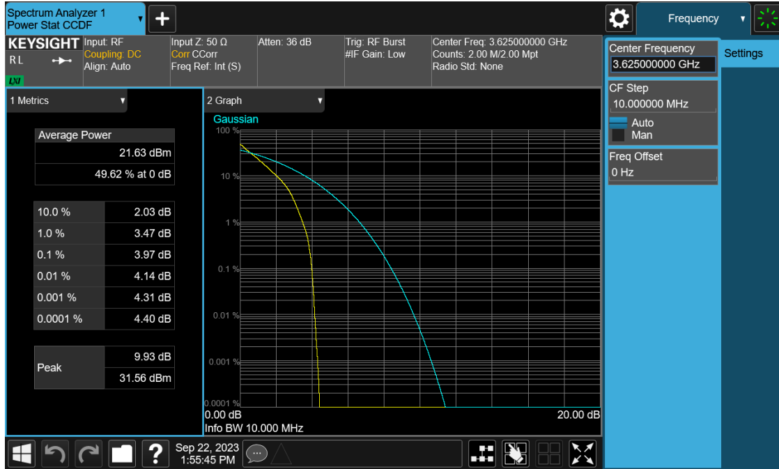
Plot 7-541.PAR Plot (NR Band n78 - 10MHz DFT-s-OFDM BPSK- Full RB)
