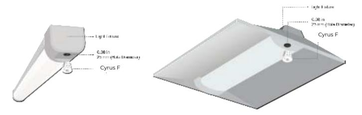
Gently insert the device in to the hole
