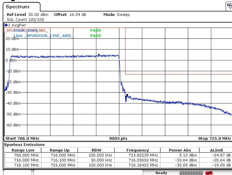
**16QAM, BW 10MHz, RB1-0****Channel: Low**
