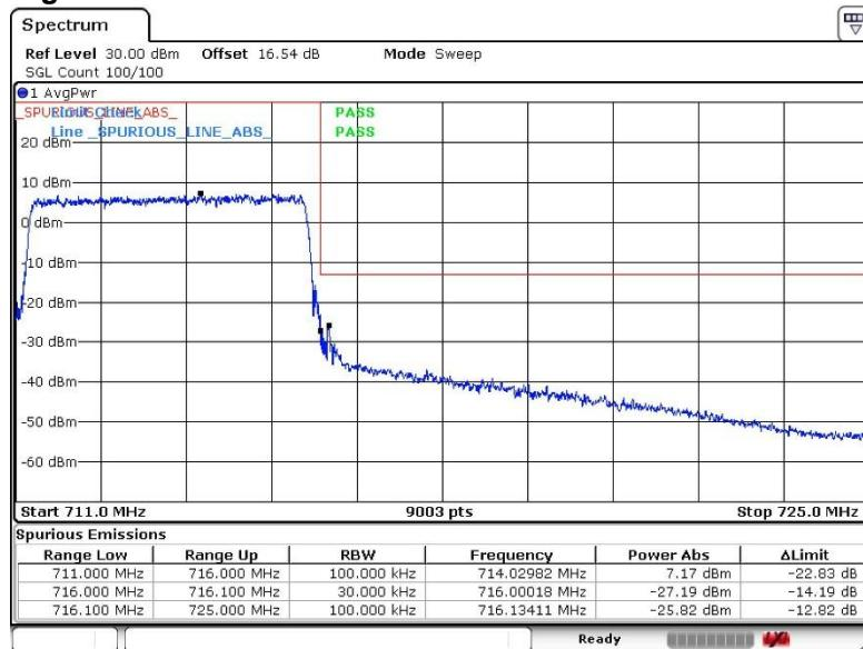
**64QAM, BW 5MHz, RB1-0****Channel: Low**
