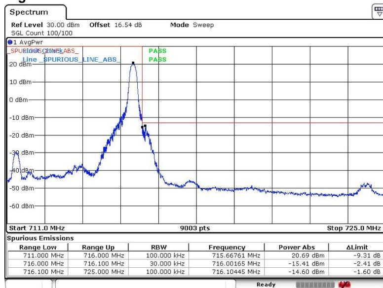
**16QAM, BW 5MHz, RB25-0****Channel: Low**
