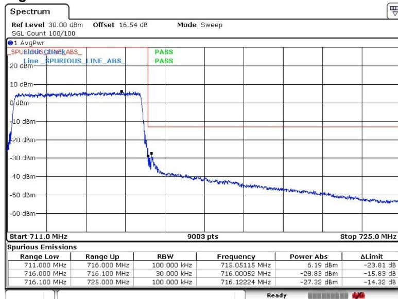
**QPSK, BW 10MHz, RB1-0****Channel: Low**
