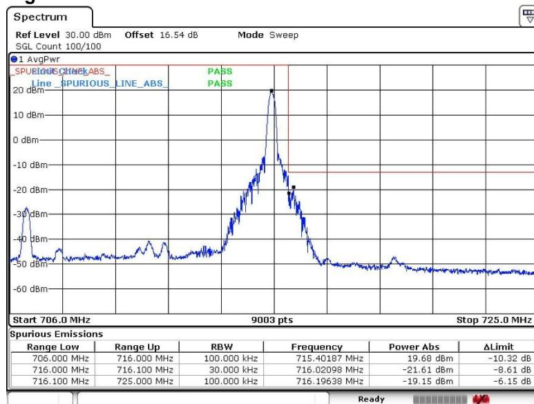
**64QAM, BW 10MHz, RB50-0****Channel: Low**
