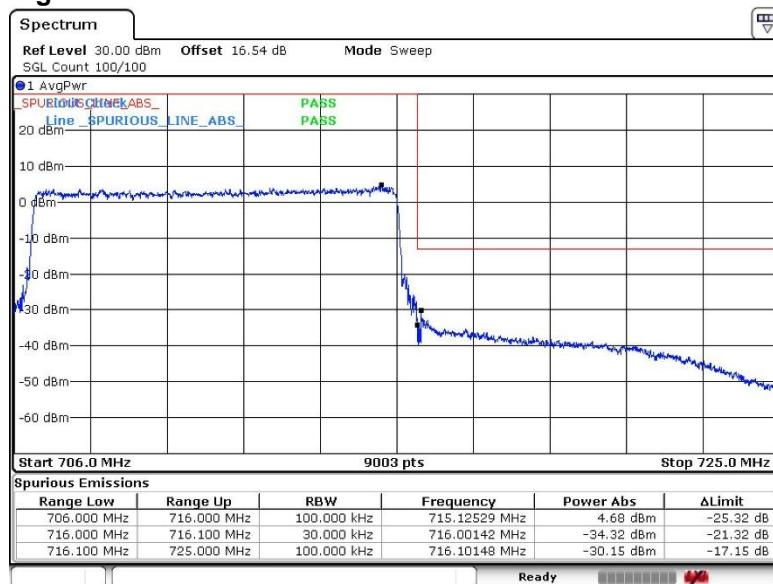
**64QAM, BW 10MHz, RB1-0****Channel: Low**
