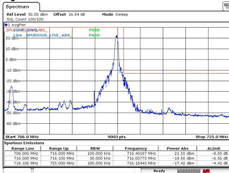
**QPSK, BW 10MHz, RB50-0****Channel: Low**
