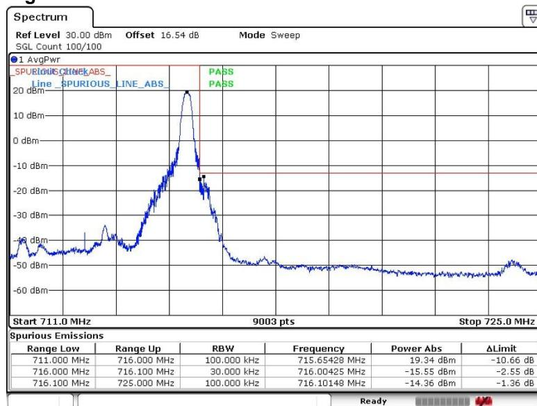
**64QAM, BW 5MHz, RB25-0****Channel: Low**
