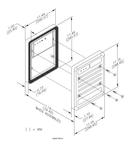
The cover is secured with four supplied screws (screw hole plugs included).
