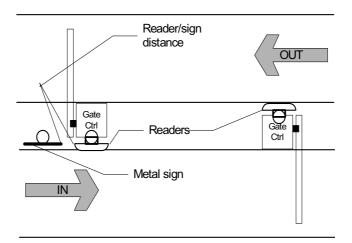
Signs and other metal objects, including hidden wiring may interfere with the reader's read field.
