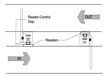
In Application A, the back-to-back and (if used) vertical gap guidelines above must be observed. Remember to mount all readers (and all other structures) before tuning the reader.
