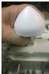
Figure 6: Attaching GPS antenna to unit
