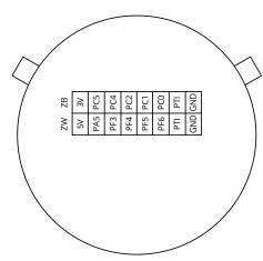
Pins in the ZB row (except for 3V and GND pins) are pins of the Zigbee/Thread/BLE EFR32MG21 chip. Pins in the ZW row (except for 5V and GND pins) are pins of the Z-Wave ZGM130S chip.
