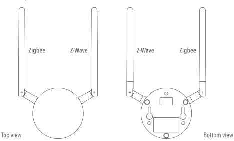
To achieve the best radio performance, make sure to always position antennas vertically and far from metal parts and cables.
