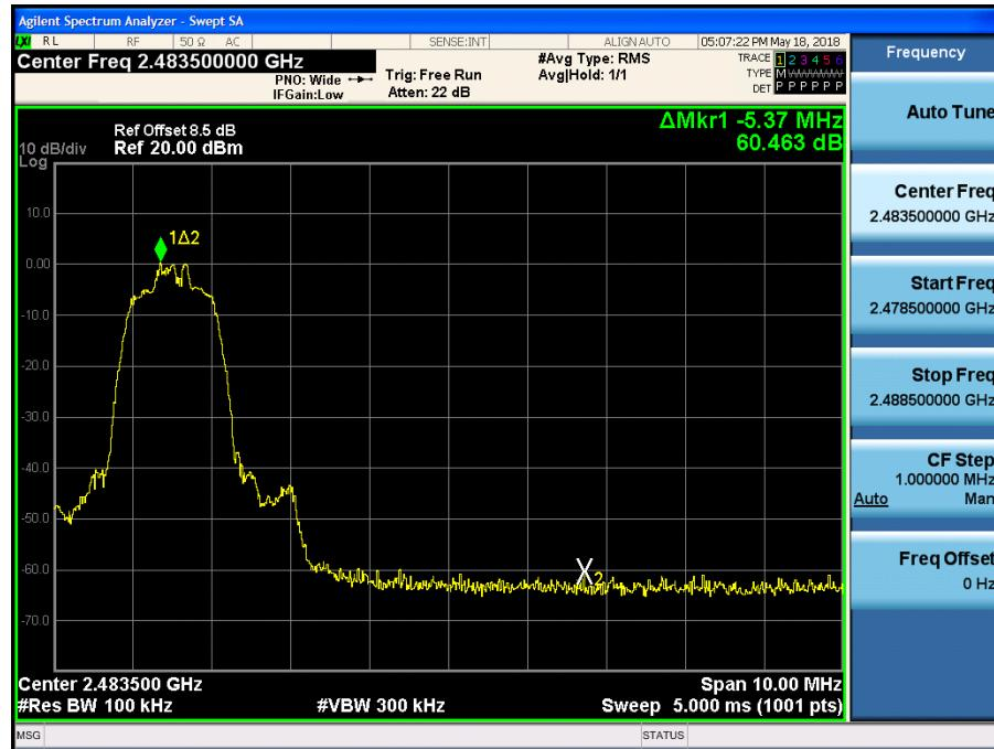
Test Plots with hopping (GFSK)
