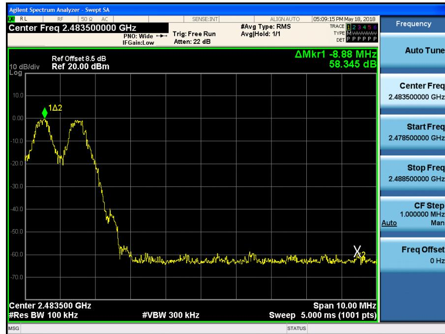
Test Plots with hopping (8DPSK)
