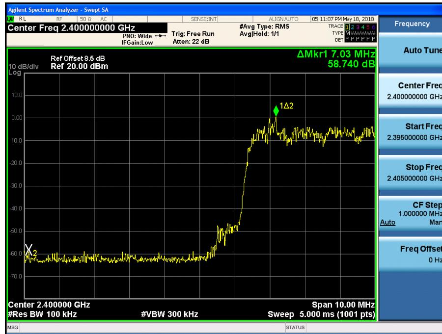
Test Plots with hopping (8DPSK)
