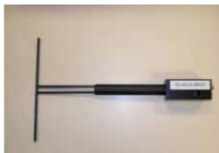
Figure 1 – Satimo COMOSAR Validation Dipole
