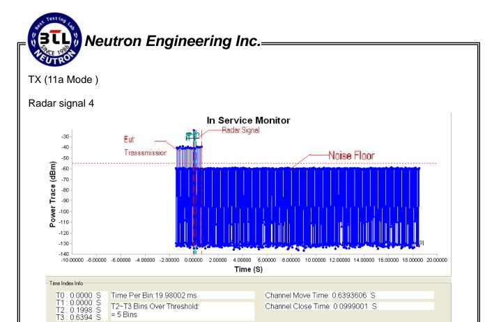
Note: T1 denotes the start of Channel Move Time upon the end of the last Radar burst.
