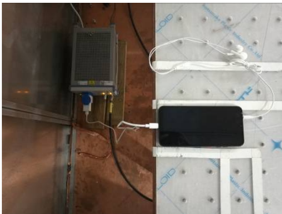
Conducted Emissions Test Setup (with charger)
