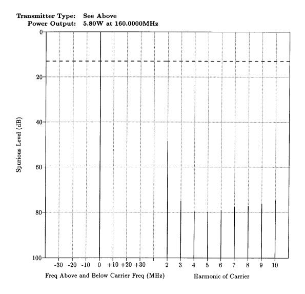
The conducted spurious level is plotted in dBm on the vertical axis. The specification for conducted spurious emissions is -13 dBm. All non-harmonic emissions are at or below the noise floor.
