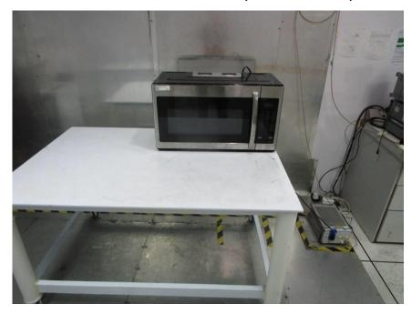
1.2 Radiated Emissions (30MHz-1GHz) Test Setup
