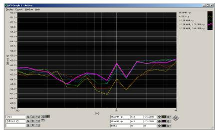
Figure 8-3 **UMTS Audio Band Magnetic Noise**
