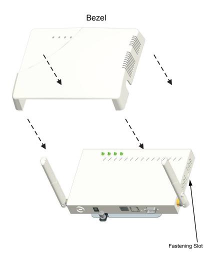
To remove the bezel, grasp both sides and gently pry away from the fastening slots located on each antenna side. Pull the bezel clear of the access point.
