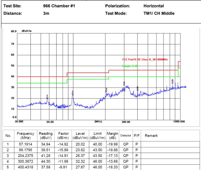
Note: Level = Reading + Factor Margin = Level - Limit
